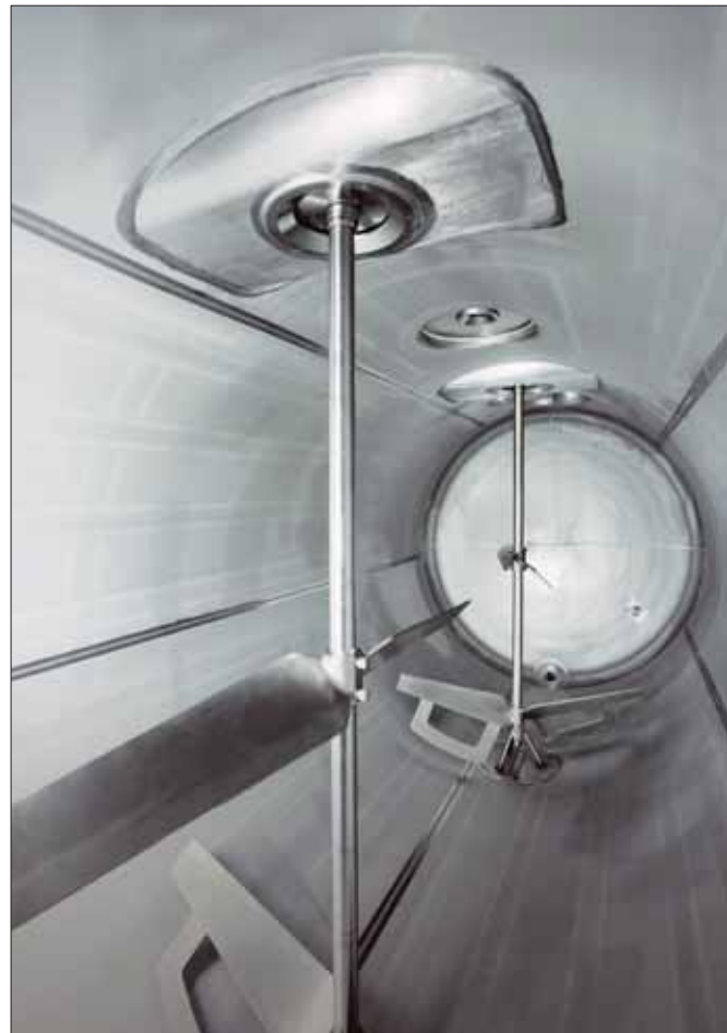
The agitators move the heated product around to ensure a constant temperature is maintained
