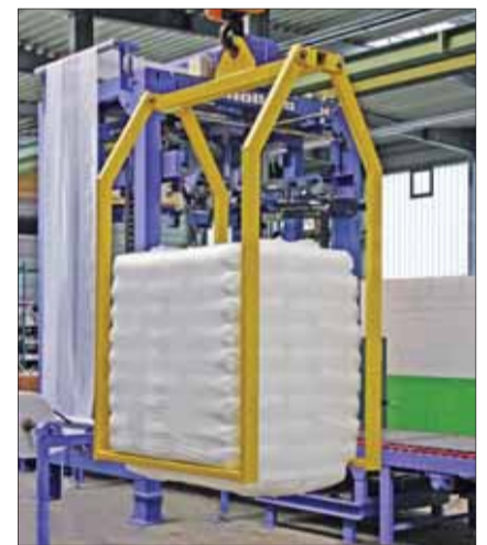
With the new Möllers reverse hood system, bag stacks can be securely wrapped with no need for a pallet and without use of heat
