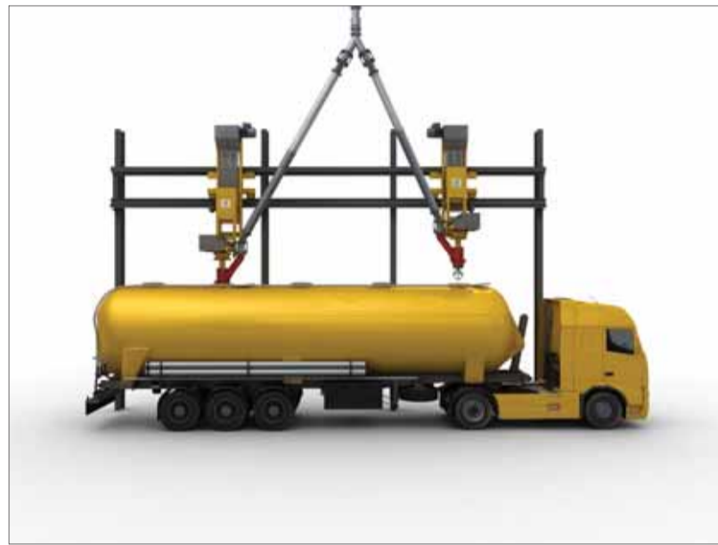
Side view of an N2 Bulk Loading System from Machinefabriek Nijsten which has lateral displacement capability; a spreader device can be seen at the lower extremity of the right-hand chute
