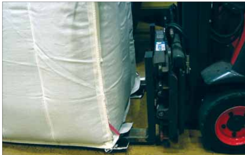
Storsack's palletless FIBC provides easy forklift entry while maximising available headroom
