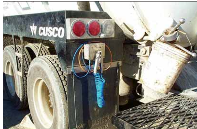
Back end of a vacuum powder tanker equipped with earthing system
