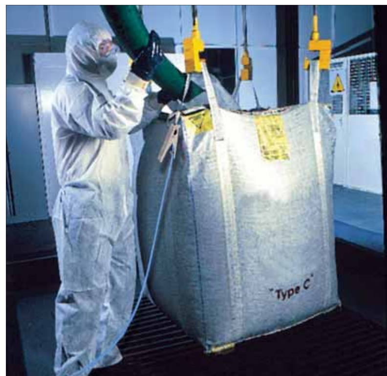
FIBC being filled with earthing clamp attached
