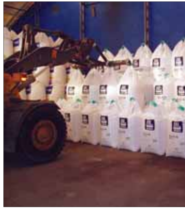
Thanks to uniform and de-aerated filling these PORTABULK single point lift bags can be safely stacked three high
