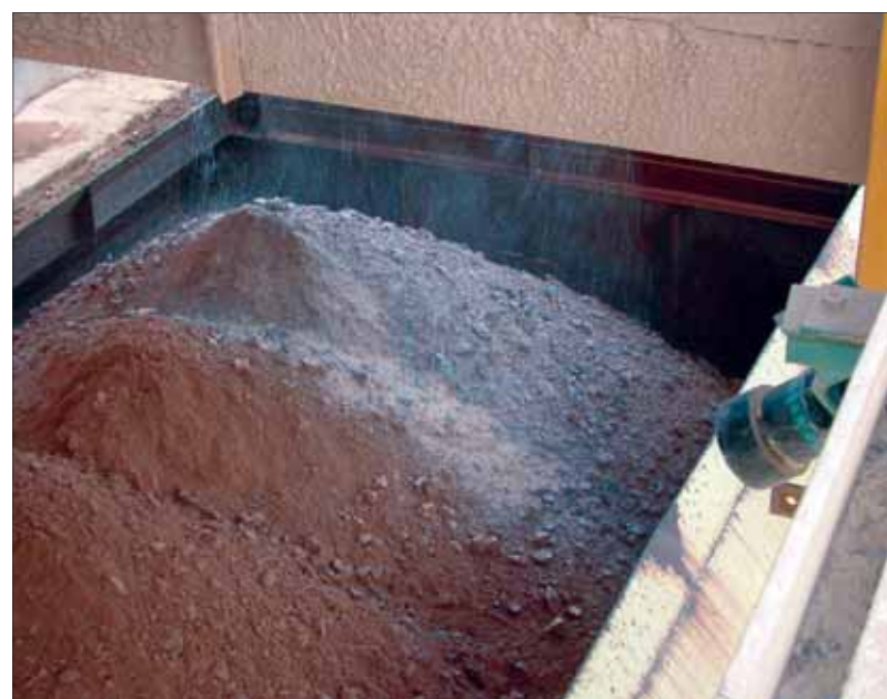
Pulsar ultrasonic device (right) controls railcar dust-suppressant spray
