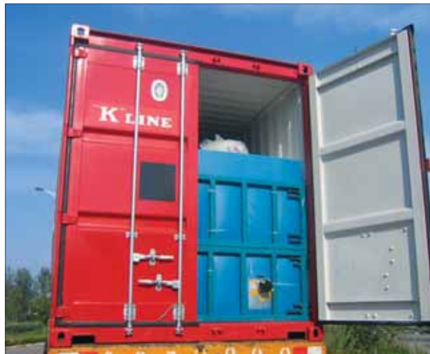
LAF manufactures flexitanks in sizes from 14cbm up to 24cbm in order to maximise the capacity of a 20ft container
