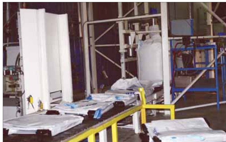
FIBCs fitted with the Drader BagPal pallet replacement system prior to being filled
