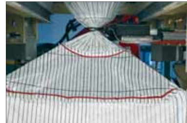
Nordenia/Reis fully automatic 4-loop bag filling system, showing (clockwise from top left): the robot picks up an empty FIBC, brings it to the filling rig, connects filling spout and attaches loops, then ties off the spout after filling
