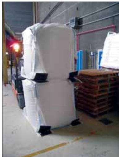
The universal pallet can be attached beneath FIBCs or other modes of packaging
