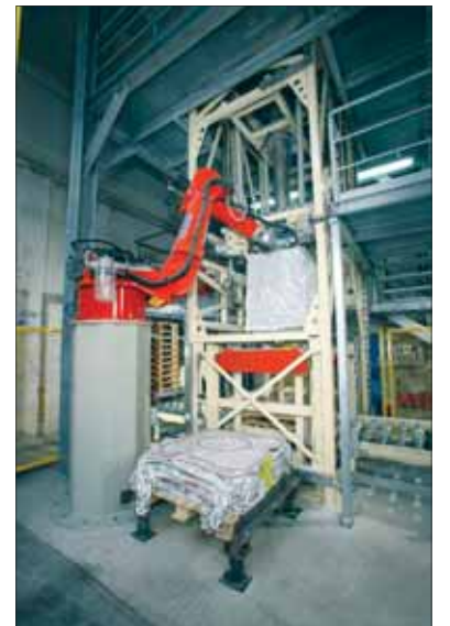
Nordenia/Reis fully automatic 4-loop bag filling system, showing (clockwise from top left): the robot picks up an empty FIBC, brings it to the filling rig, connects filling spout and attaches loops, then ties off the spout after filling
