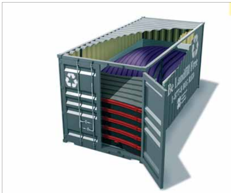
The Wine-Pac's construction features an outer woven layer of polypropylene specially woven with 'strength bands' running the length of the bag
