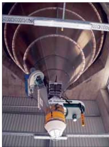
Gravity discharge directly into bulk containers or road powder tankers can be achieved by means of Cimbria Moduflux telescopic loading chutes
