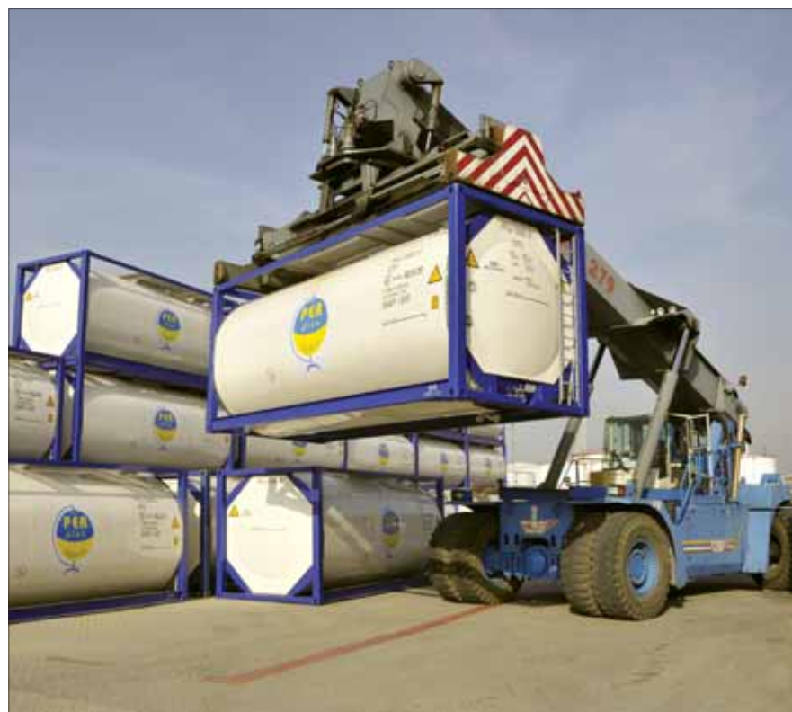
The PER Plus fleet has now grown to over 300 units. The standard specification of its own tanks is the 26,000 litre type IMO/ADR T11 single compartment unit
