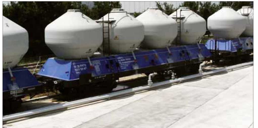
Last year Gericke installed a specially adapted positive-pressure pneumatic conveying system at Transportbeton in Vienna for unloading cement from rail tankcars to silo storage
