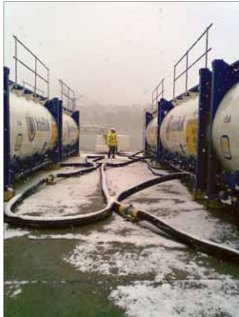
An important safety advantage of ISO-Veyors is that, unlike with traditional vertical silos, there is no need for a person to climb on top of the structure to perform certain operational or service tasks
