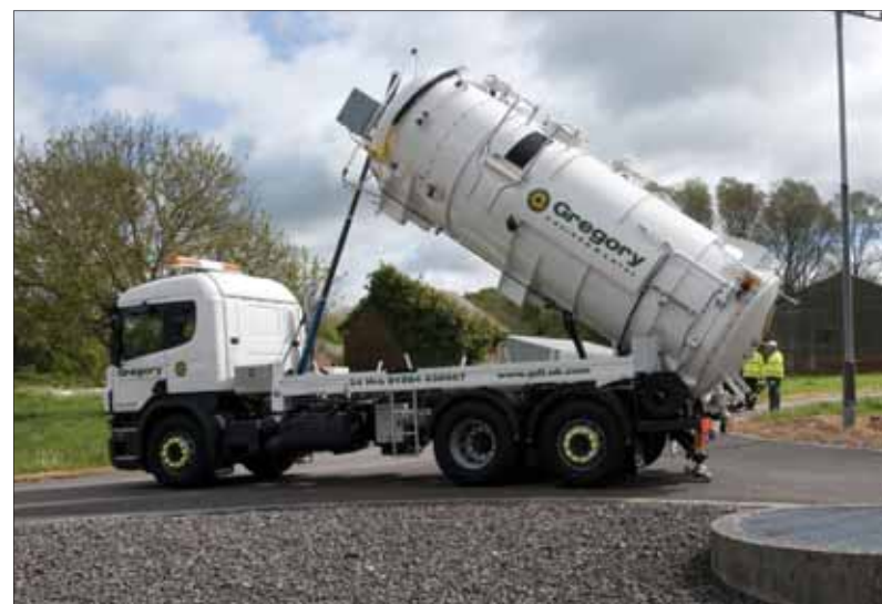
Two Whale tankers have joined the fleet of Gregory Environmental Services. Pictured is the larger of the two new units, which features Whale's 3,200-gallon capacity carbon steel vacuum tank mounted on a Scania P310DB 6 x 2 26 tonne chassis
