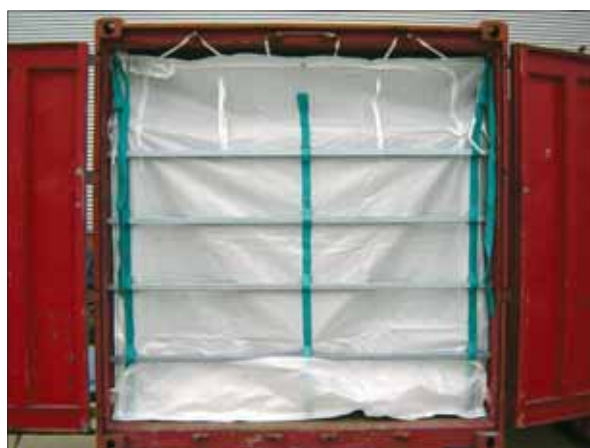
40ft woven PP liner from Ligtermoet, the Netherlands, provided with zipper closure and ready to be loaded
