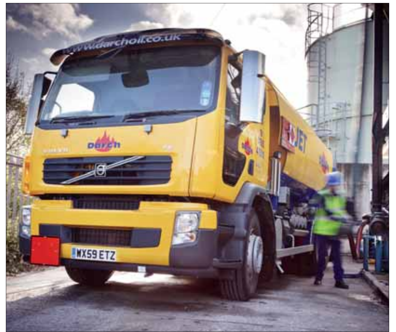
The 6x2 tanker combines the manoeuvrability needed for access to small premises and rural roads with the payload essential to generate economical delivery
