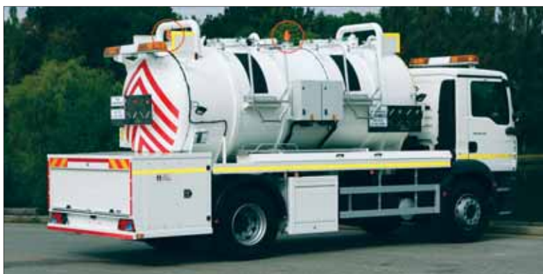
The Hycontrol onboard radar level system provides a safe measuring alternative to working at height
