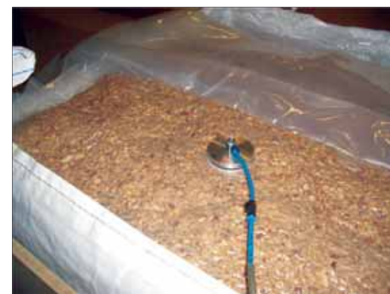
A vacuuming compressor working in conjunction with a patented liner valve are the key elements of BT-Pack's new concept
