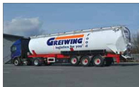
New Greiwing powder tanker used exclusively for transporting foodstuffs
