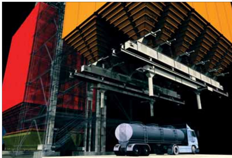
Two road tankers can be loaded simultaneously at the Wozniak silo complex
