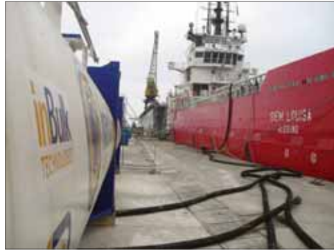
The ISO-Veyors are capable of providing high-capacity and totally enclosed transfer of bentonite and barites to the rig supply boats
