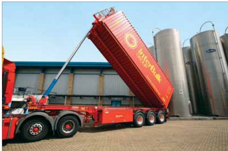
Containerised bulk goods being delivered directly to the customer's vertical silo facility
