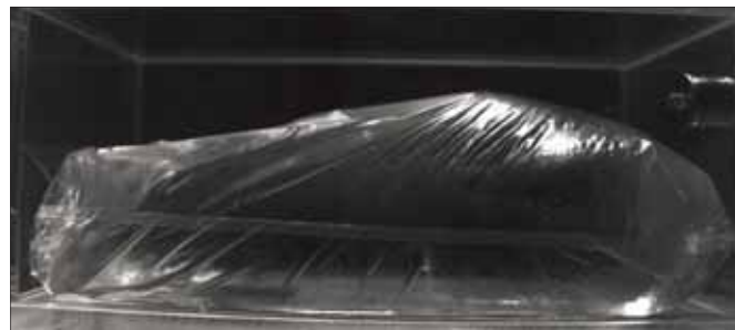
Model-scale flexitank rail impact testing
