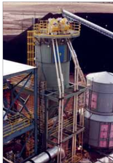
Spiroflow's Cableflow tubular cable drag conveyor suitable for delicate products and right multiple installations of the heavier-duty Dynaflow tubular chain drag conveyor shown here feeding a silo.
