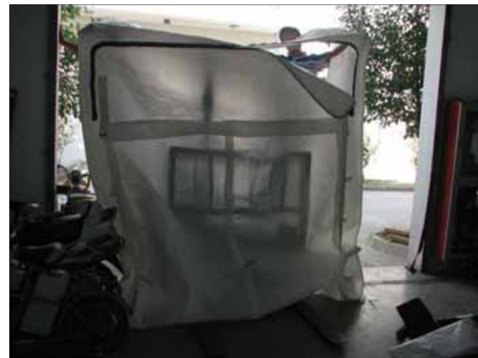
For one of its customers B Pack has devised a special frame to secure the liner inside the container without need for double-sided tape
