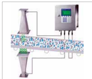
Operating principle of Berthold Technologies Micro-Polar moisture measurement system.
