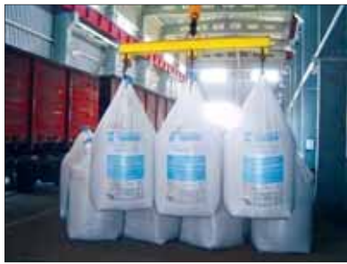
Chempack single-point-lift FIBCs handling salt
