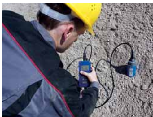
Left: measuring the moisture content of sand and right: in its robust carrying case
