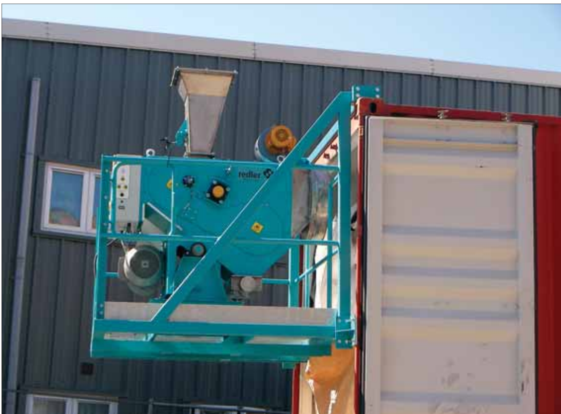
Redler FulFiller shown attached to the back of a container
