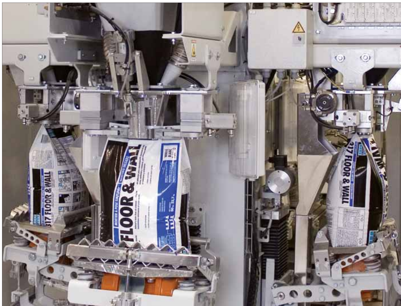
Haver & Boecker ADAMS 2000 technology for environmentally friendly filling of powder-type products into watertight PE bags
