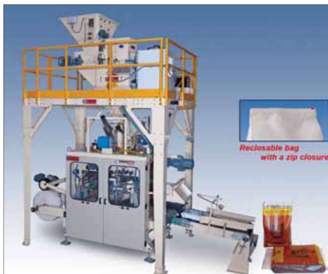
Concetti FFS bagging machine showing a zip-closable bag inset
