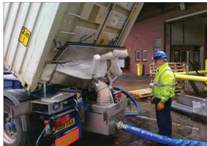
Carl Schmidt Group has recently begun using specially designed food-grade liners for containerised transport of sugar see p3 for further details
