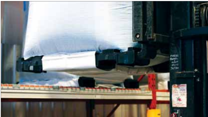
Racks support the BagPaliT which in turn provides a secure saddle to support the filled FIBC. The base of the FIBC does not come into direct contact with the rack
