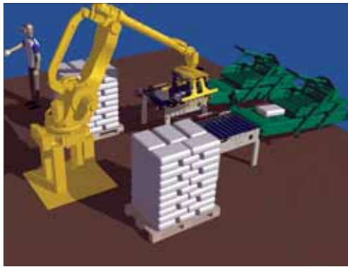
Model of one of Newtec's new robotic bag palletisers and right the versatile gripping tool
