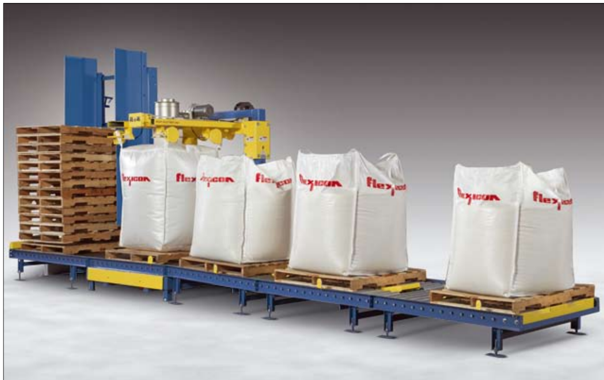
Bulk Bag Filling Line: a 15-pallet dispenser releases the bottom-most pallet to roll beneath the cantilevered fill head of the bulk bag filler. Following manual connection of empty bags to the fill head, filling, densification and conveying functions are automatic
