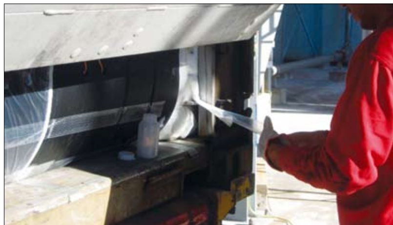
Eceplast Safety Liner with patented anti-bulging system. The liner allows the driver to sample the product from the letter box and eventually reclose it in case of product rejection while avoiding exposing personnel to unnecessary risk of injury
