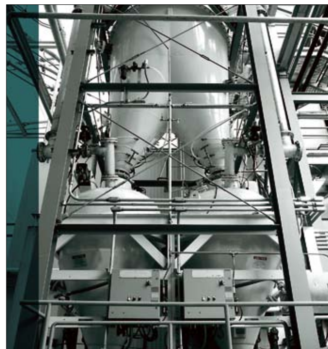
The loading stations feature a modular design and have a number of options for unloading sacks, bulk bags and octabins
