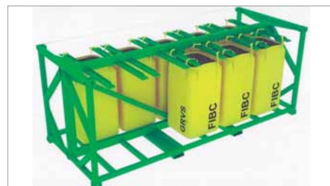
The special suspension frame is fitted with 10 sets of forks from which the FIBCs are suspended. These forks have a central channel slightly wider than the blades of a forklift truck. For loading, the forklift operator merely has to insert the blades, from which the FIBC is suspended, into the twin channels and withdraw, leaving the bag suspended from the frame's forks. For unloading the same process is repeated in reverse.
