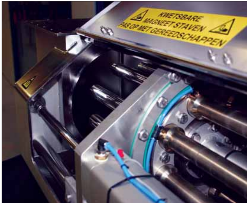
www.goudsmit-magnetics.nl Enhanced Goudsmit rotating clean-flow magnetic is suitable for other food products such as cocoa powder
