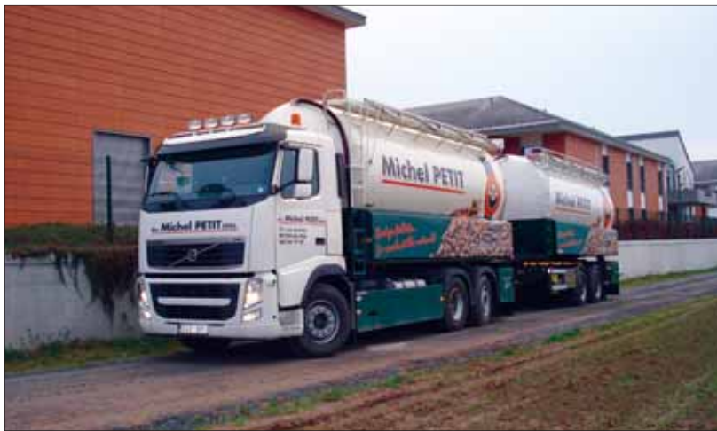
The Michel Petit trucks are equipped with electrostatic protection in contact with the ground to avoid risk of explosion
