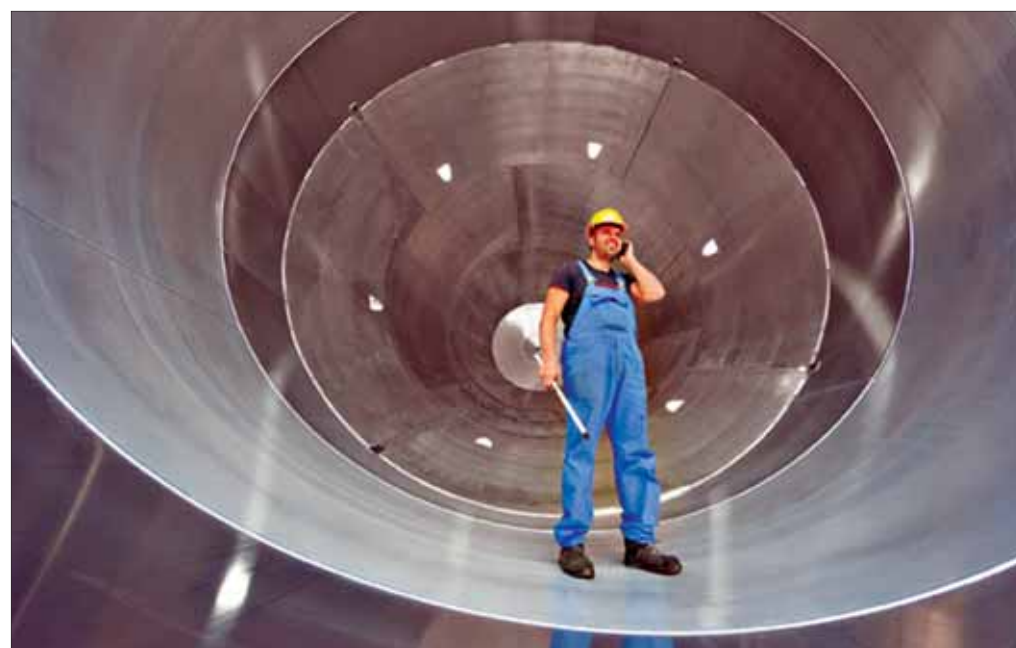
Zeppelin's Panel Tec silo concept involves modular construction, bolted assembly and internal welding
