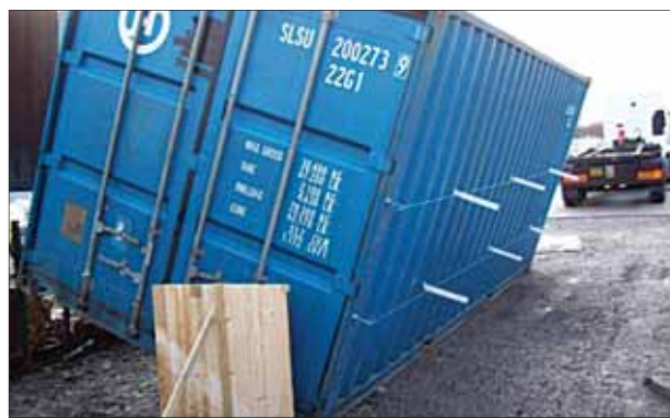
Fig.3 Container successfully undergoing 25% tilt test in Manchester, December 2008
