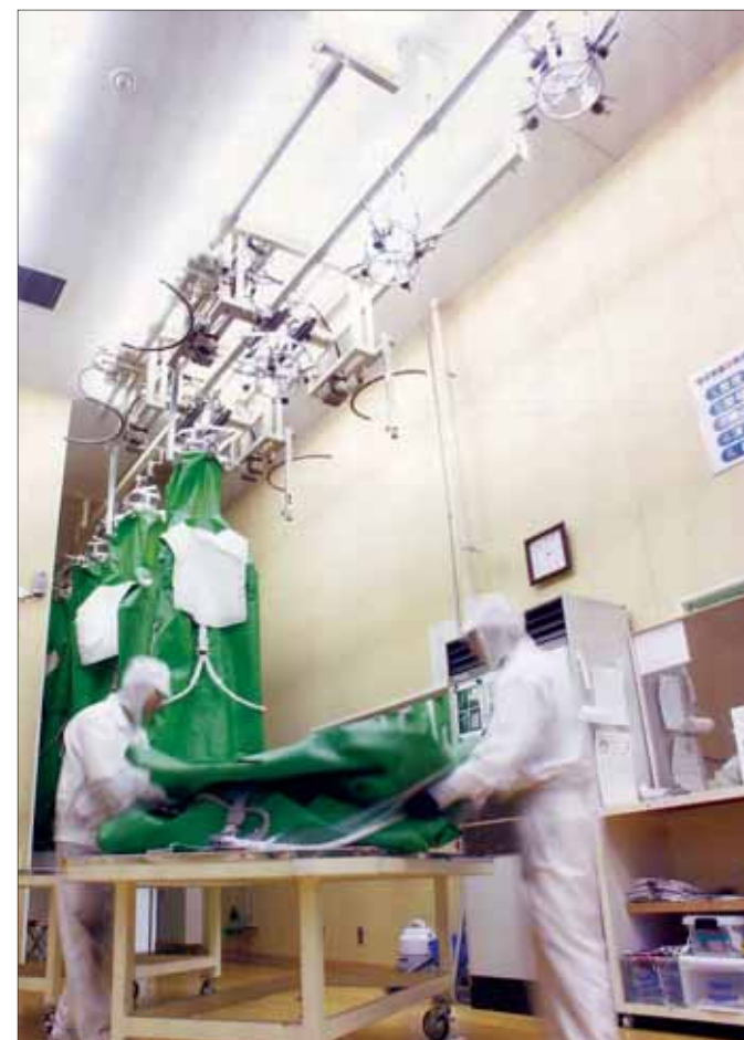
Taiyo Kogyo bag being folded for delivery back to the customer after being washed; unlike PP fabric FIBCs, this type of big bag does not shrink as a result of wet cleaning
