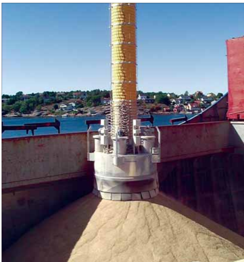
Moduflex loading chute from Cimbria Bulk Equipment, showing fully self-contained integrated filter modules on the chute outlet
