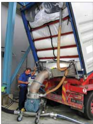
TBMA Europe which engineers systems for pneumatic discharge of containers emphasises the importance that air leakage, line pressure and rotor speed should be properly balanced
