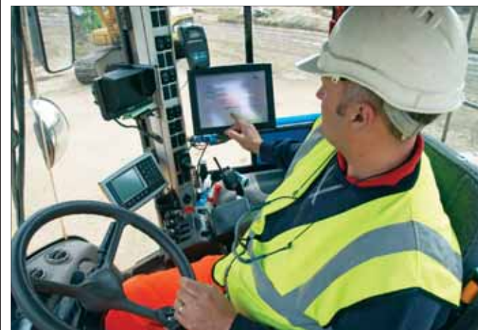
In-vehicle PC is used to weigh vehicle loads without the need for a weighbridge
