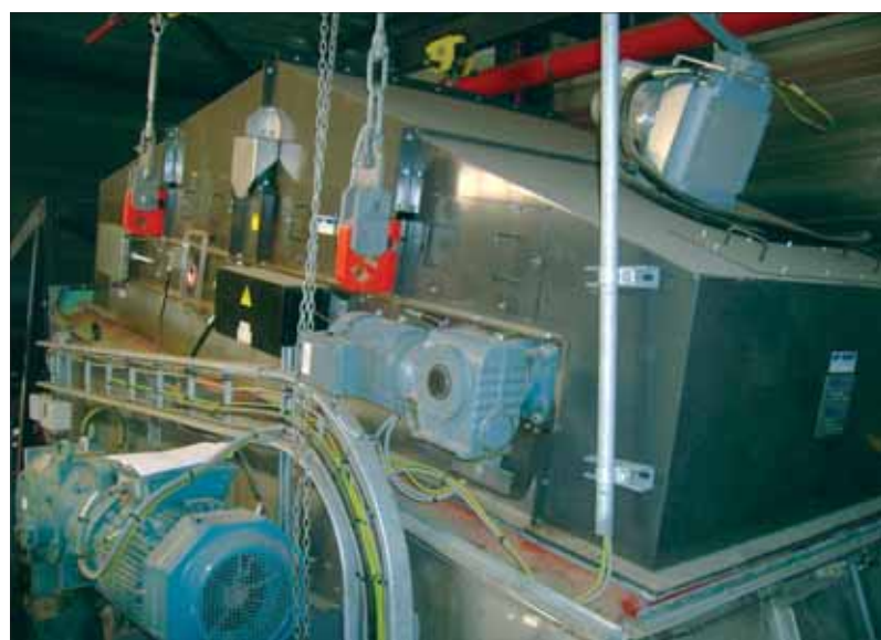
Goudsmit ATEX-compliant overbelt electro-magnet
