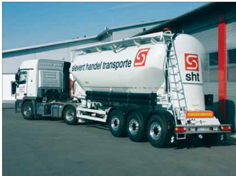
Typical SF-Series non-tipping type semi-trailer from Spitzer offering a payload of around 30t
