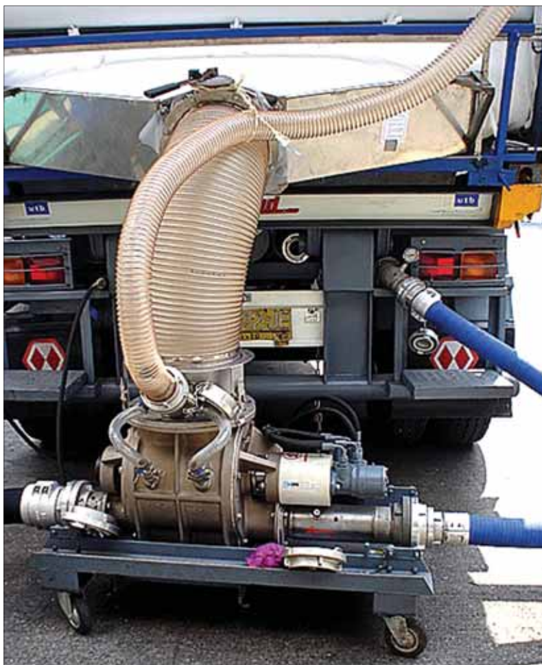
Mobile TBMA rotary valve discharging granules from a container
