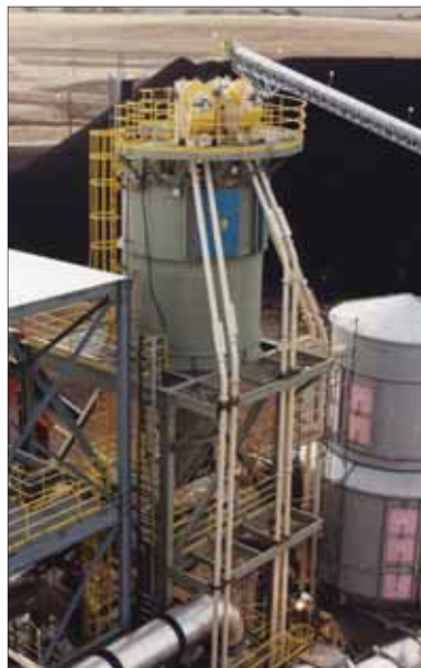
Dynamet tubular drag conveyor system delivering material to a silo; the equipment will soon also be available in Europe
