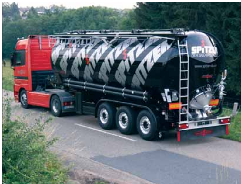
Spitzer SK 2745 CAL tipping semi-trailer with a total length of 9.825m, volume of 45m 3 and payload capacity of about 28.5t
