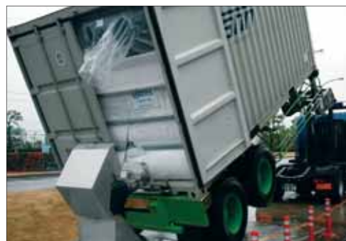
The Caretex safe discharge method, with one door kept closed and the container tilted at an angle of 28 degrees
