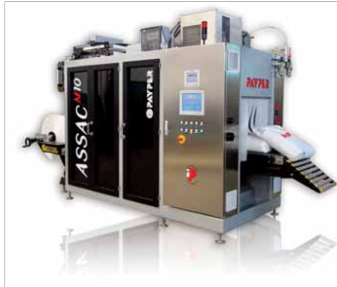
The ASSAC M10 FFS bagging system from Payper, Spain, can achieve outputs up to 2200 bags/h
