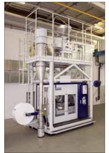
DELTA NT (New Technology) is the latest Haver & Boecker mobile FFS system for filling free-flowing loose products
