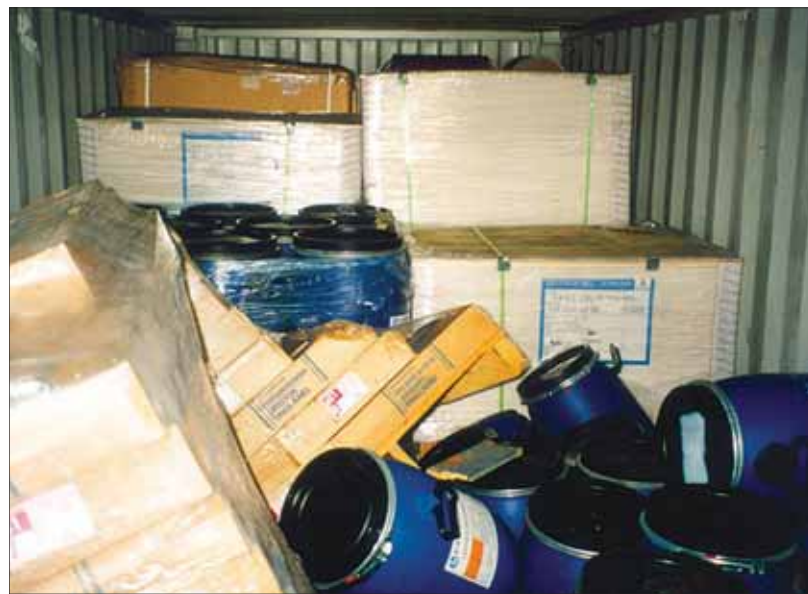
There are safety issues when loading drums into a dry container
