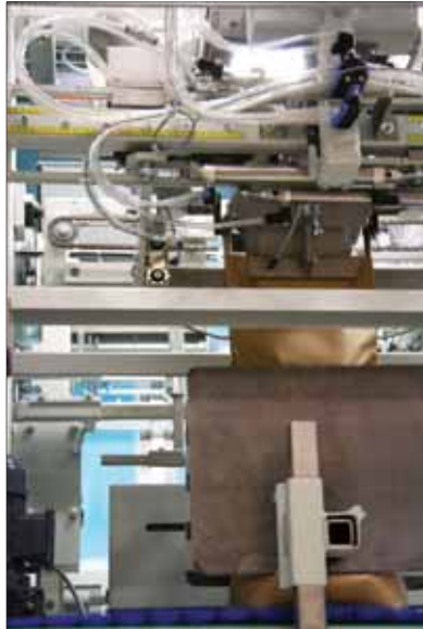
Novel dust-free bottom-up filling technology
