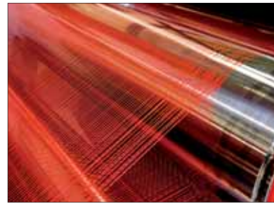
Tapes running over godets on a Starlinger starEX tape extrusion line of the type delivered to the new UAC plant in Jeddah
