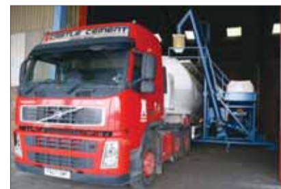
Guttridge's bespoke road powder tanker loader
