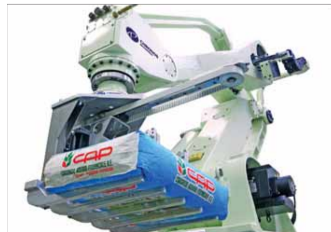
The upgraded CHRONO-PAL RP robot palletiser can now handle up to 1200 bags/hour from a single bagging line.
