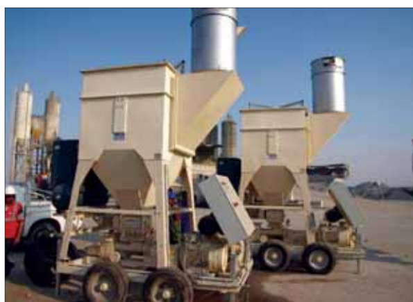
Telschig mobile bulk bag unloading rig, designed for discharging cement and similar materials
