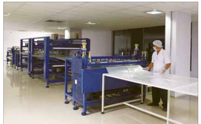
Liner sealing machine
