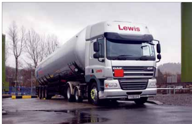
Using 17.5 ins wheels on the mid-lift axle has reduced the weight of the tractor by around half a tonne
