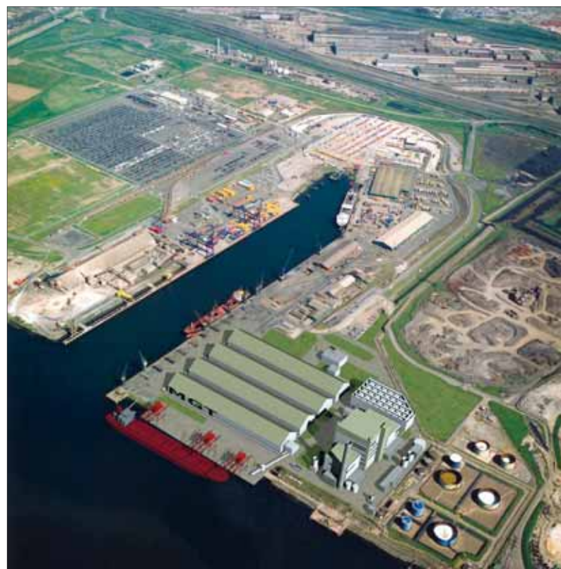
The new berth will accommodate vessels up to 240m long and 38m wide
