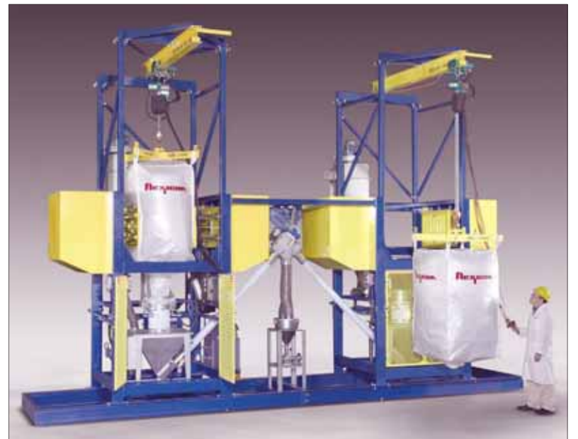
With this novel Flexicon arrangement, dual bulk bag unloaders are each equipped with integral conditioners to ensure steady and complete discharge even when material has become compacted.
