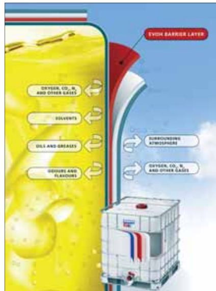
Schuetz IBCs with the EVOH permeation barrier eliminate the risk of explosive compounds arising.
