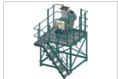
Support structure for fixed installation loading
