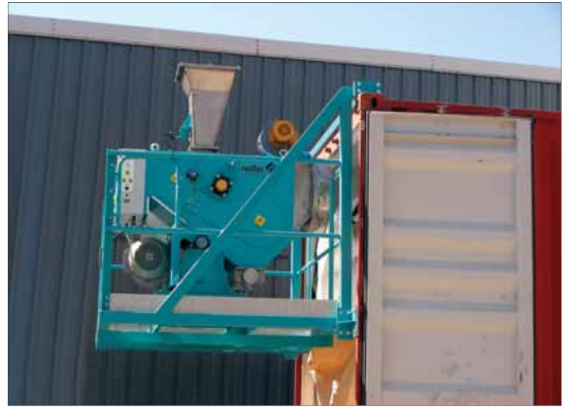
FulFiller hooked on to the rear of the container to be loaded
