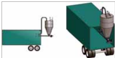
Loading by pneumatic transfer
