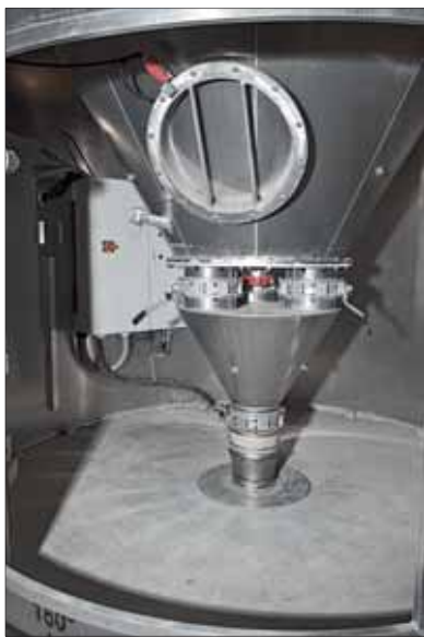
Discharge port of a blending silo which is equipped with a vertical screw designed to provide a high degree of product homogenisation
