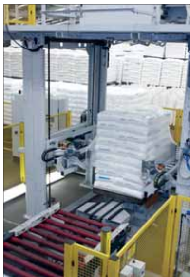
At the LyondellBasell Australia polypropylene pellet plant, a Beumer stretch-hooder applies a film hood to palletised bag stacks, which effectively protects them against the weather as well as against dust and moisture
