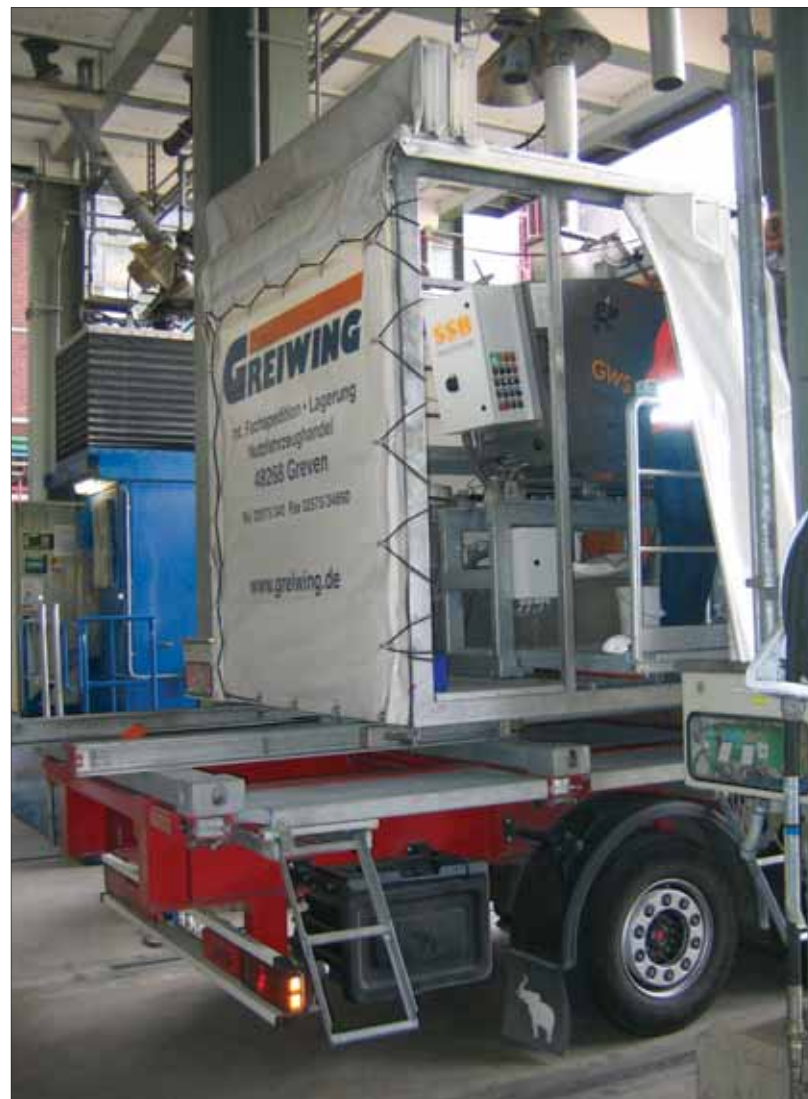
Bulk containers can be loaded through the rear door by a truck-mounted belt thrower which is easily moved into position beneath the designated silo outlet
