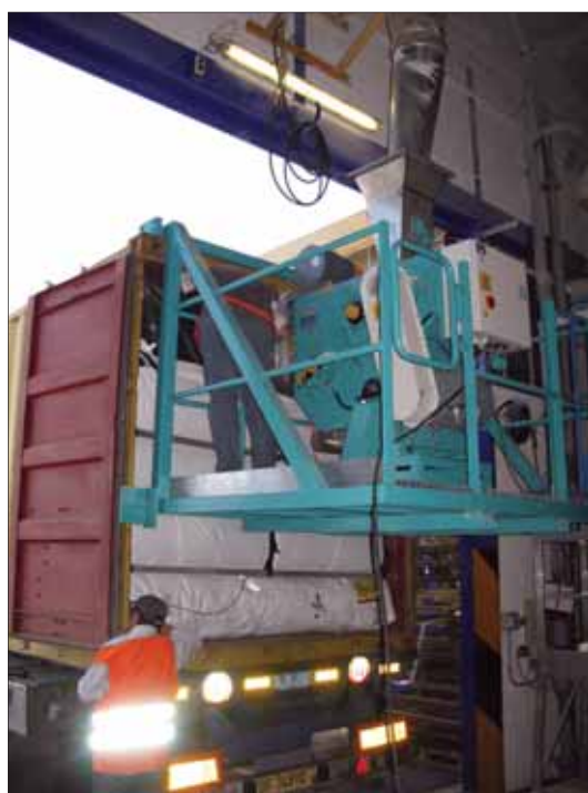
This Redler MFF type FulFiller supplied earlier this year to an Italian plastics producer is capable of loading 19t of polymer pellets in just eight minutes with minimal product attrition.
