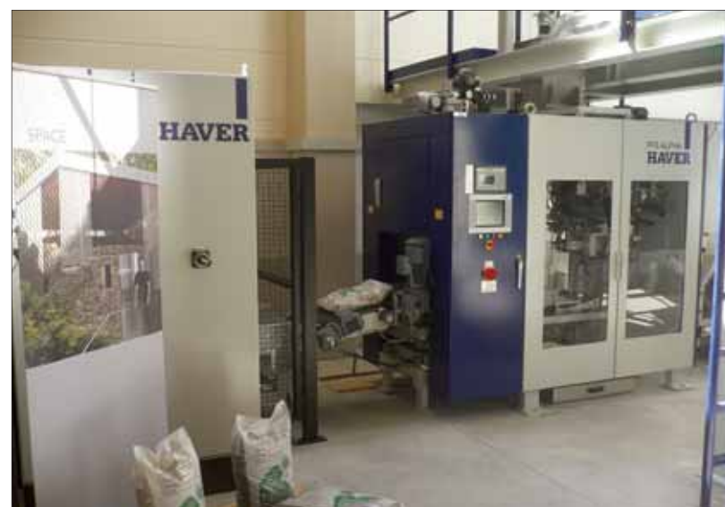
At Gandl Natursteine GmbH many different categories and sizes of stone are automatically filled and packed into film packaging by a Haver FFS Alpha machine
