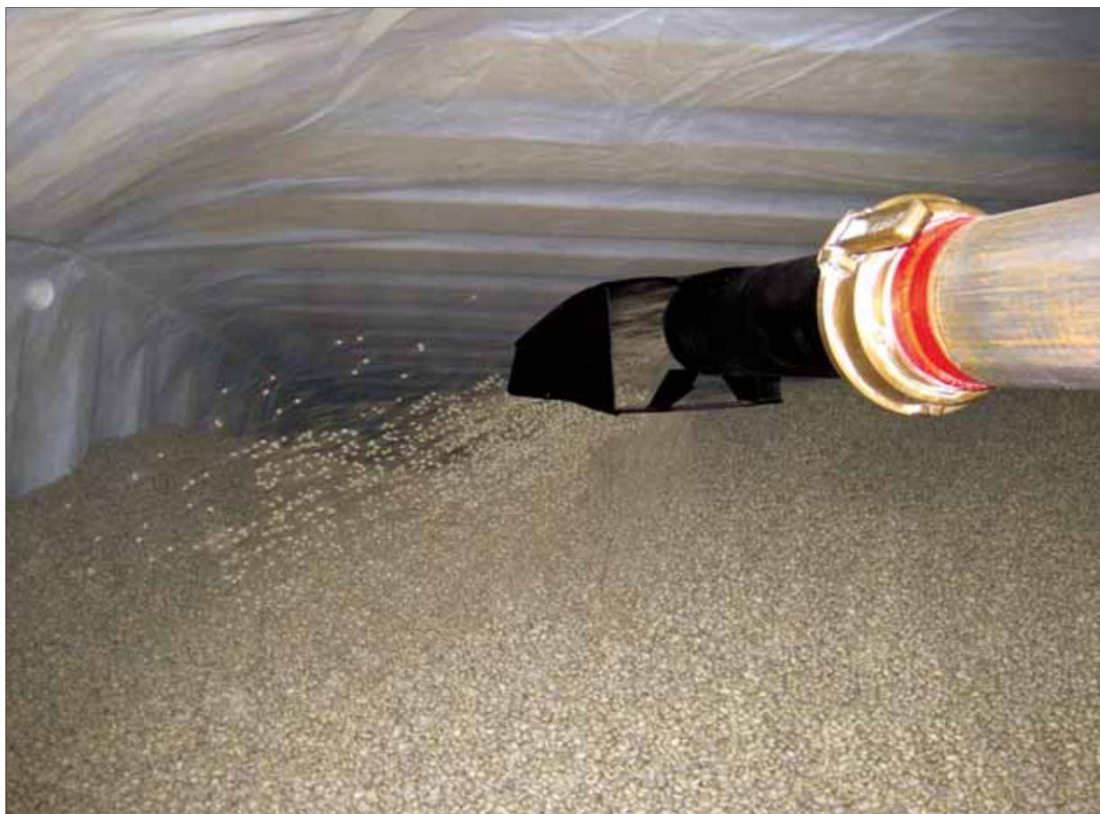
The telescopic filling pipe is a key feature which ensures complete filling of the container
