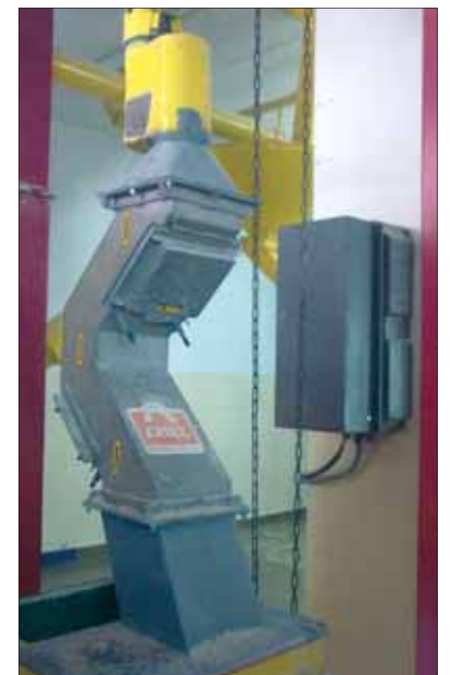
Eriez magnetic hump separator at Granexport showing (left) how it works
