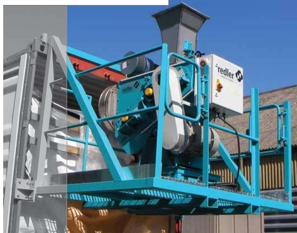
This Redler MFF type FulFiller supplied earlier this year to an Italian plastics producer is capable of loading 19t of polymer pellets in just eight minutes with minimal product attrition.
