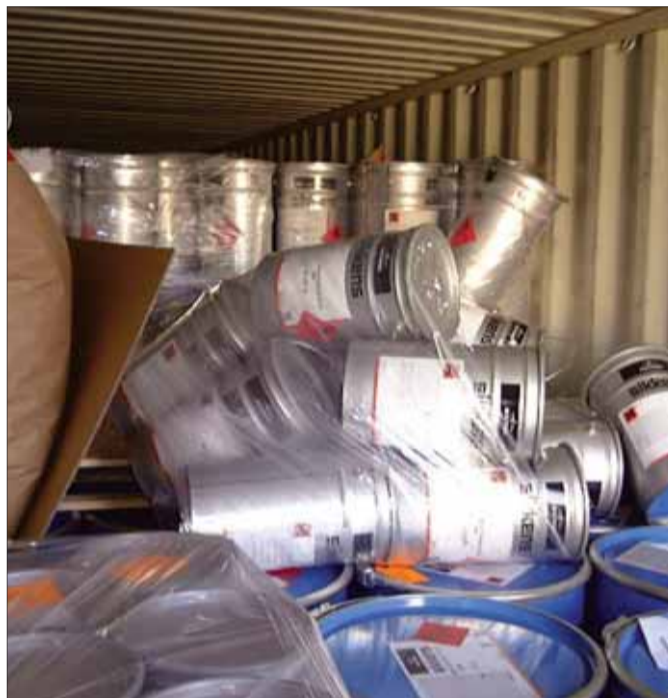
Example of a badly packed container
