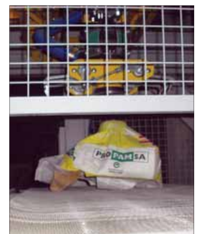
Part of the TMI automatic de-palletiser showing removal of emptied and slit bags
