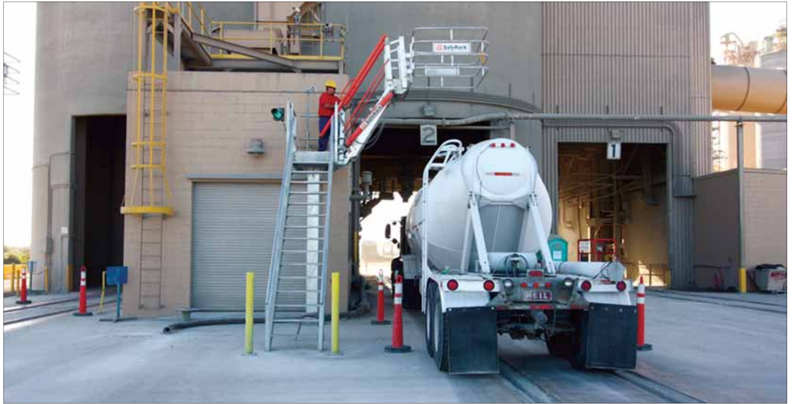
The SafeRack gangway gives operators freedom to work on top of the truck while providing safe access and fall protection
