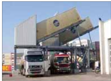
At its Vienna site Schmidt has developed a new design of dry bulk container tipping installation which can discharge two boxes simultaneously
