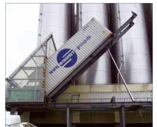
This dry bulk container tipping frame at Schmidt's Cologne-Niehl distribution centre is capable of loading railcars as well as road tankers. A similar installation is currently being built at Duisburg's Rhein-Ruhr Terminal
