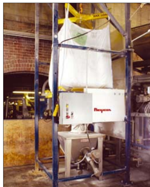
Flexibility of conveyor line routing allowed The Plastics Group to position two Flexicon bulk bag dischargers in restricted spaces, eliminating the need for a costly network of pneumatic lines.
