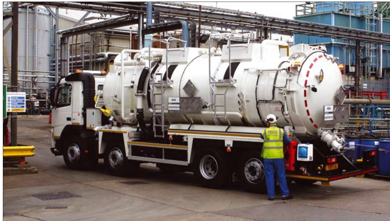
The Whale tanker was manufactured to meet full ADR class 3 regulations
