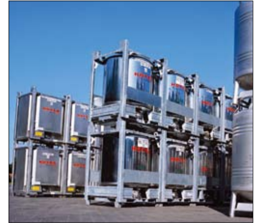
Hoyer IBCs can be supplied with special coatings, with heating, suitable for dangerous goods or liquid foodstuffs
