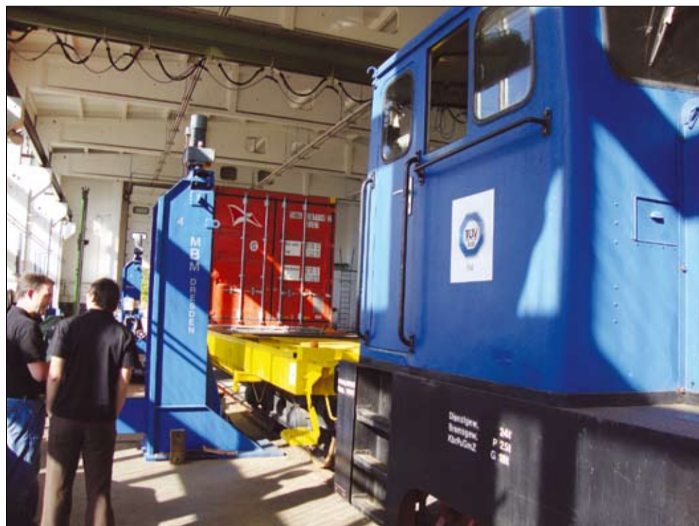
Braid flexitank being tested at Tuv Goerlitz rail test centre
