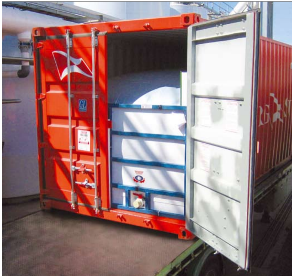
Braid BD Wine Flexitank with integral aluminium foil barrier
