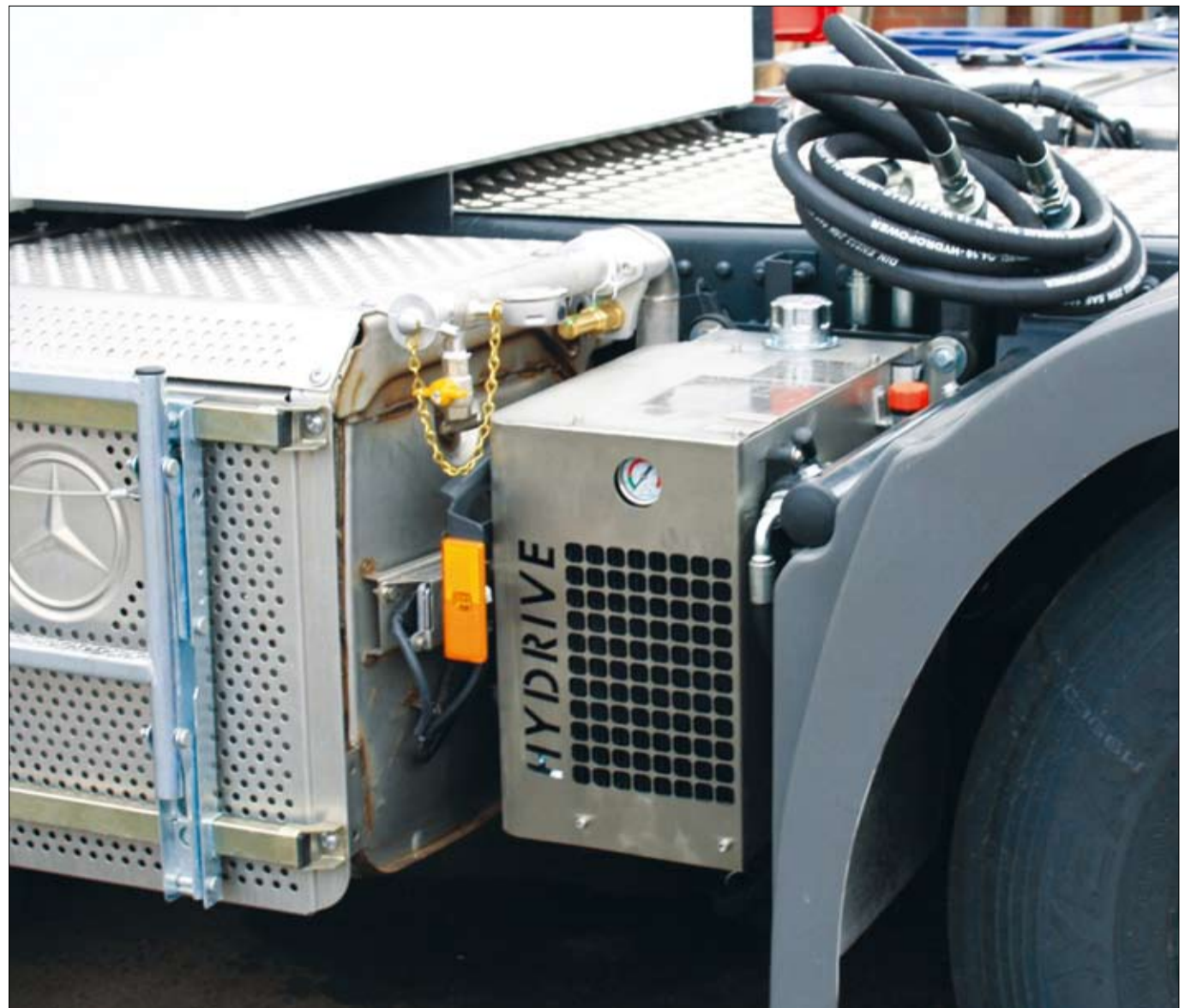
The B200 can be installed as a direct mount, with a PTO, or with a hydraulic drive.
