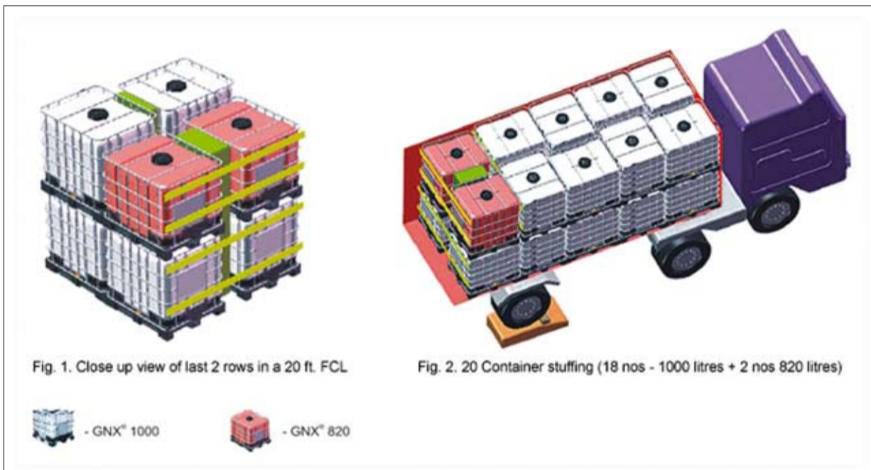
Time Technoplast's GNX 820 litre IBC can be used to stuff the last 2 slots in a 20ft container allowing up to 1,640 litres of additional product
