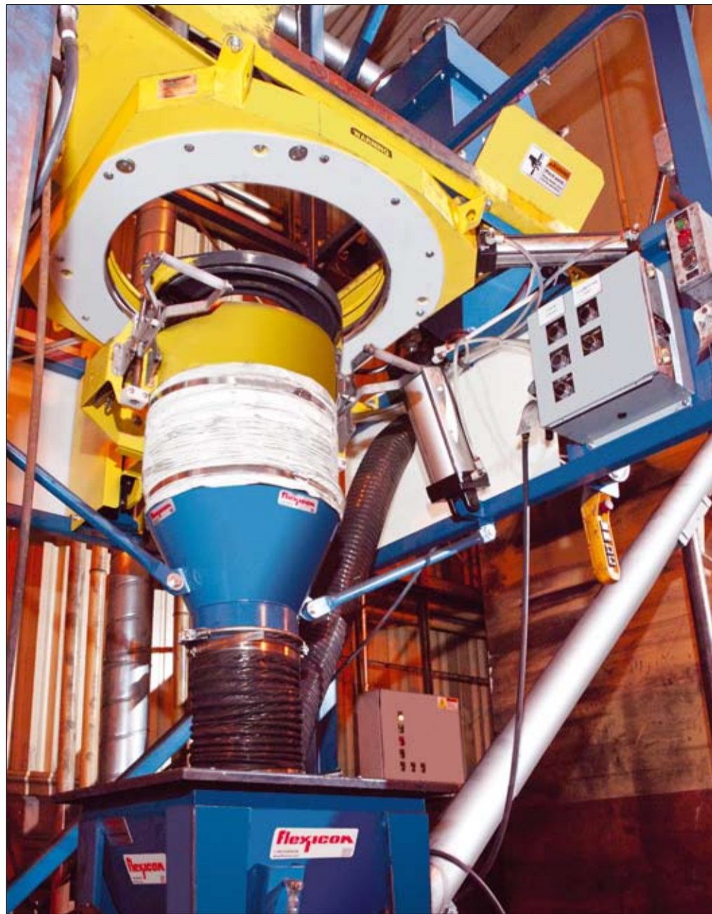
The Flexicon bulk bag discharger, hopper and flexible screw conveyor fully contain carbon black pellets, preventing dust from entering the plant environment
