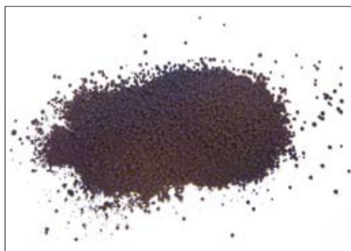
Dust is created as 1-3 mm diameter carbon black pellets rub together.
