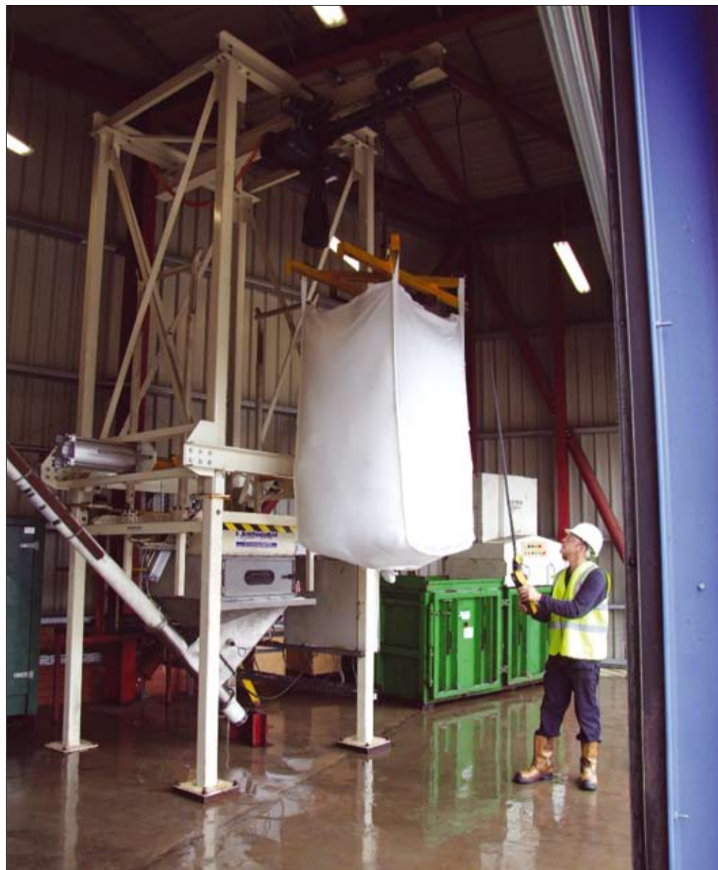
FIBC being hoisted into the Spiroflow discharger
