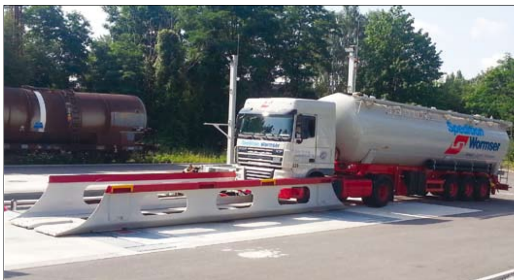
Semi-trailers are placed onto special loading pallets without the train being present, so drivers don't need to wait for trains or cranes
