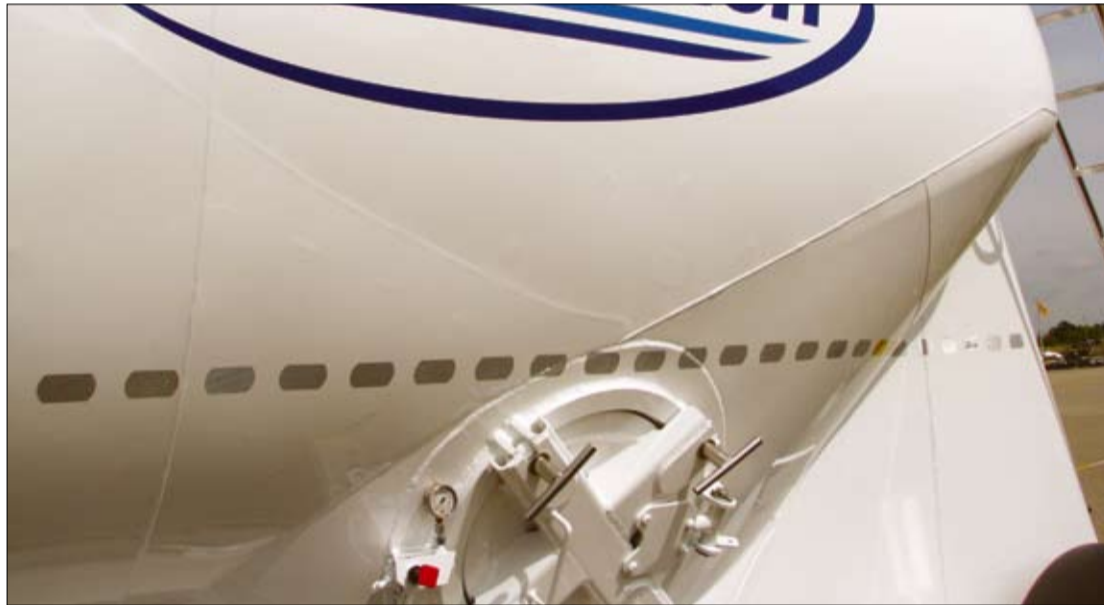
Entering the silo tanker via the side access point is still classed as entry into a confined space, but it has significant reduced risk potential due to it being near ground level
