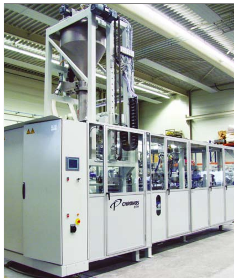
Chronos BTH OML-130 BF single spout bagging system prior to despatch from the European manufacturing facility
