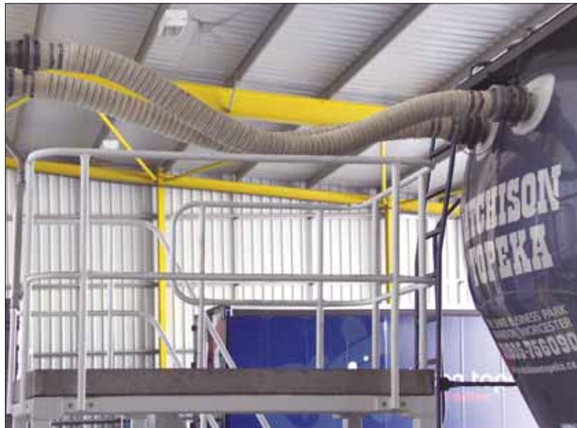
One pneumatic line discharges into the tanker's inlet port, while a second line vents an outlet port, leading to a filter receiver where dust is separated from clean air vented to the atmosphere
