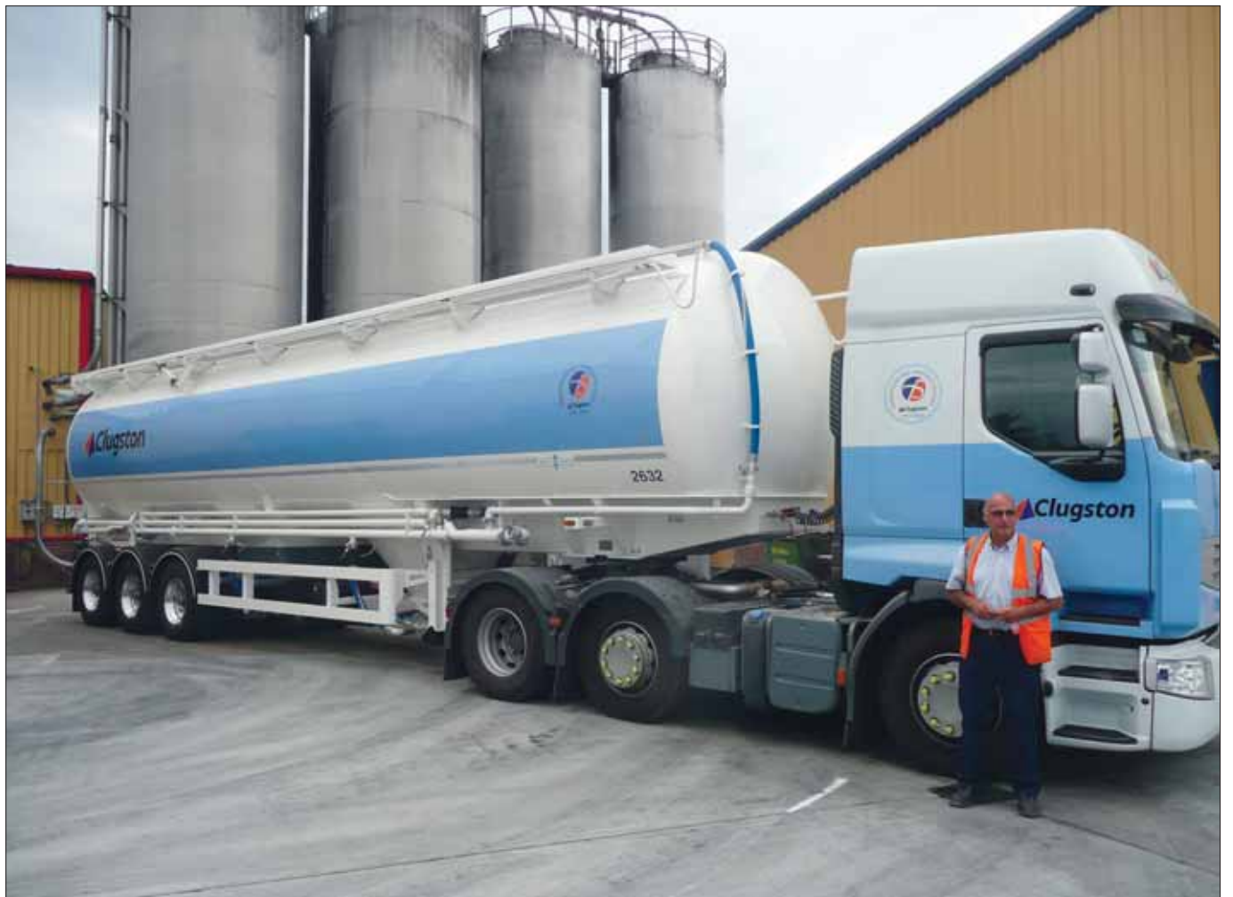
Investment also included two new Spitzer Eurovac bulk powder tankers; a food grade 60 cbm tipping silo and here a 56 cbm 4 pot non-tipping tanker
