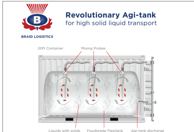
The Agi Tank uses a series of injection points in the top surface to agitate and mix the cargo pneumatically
