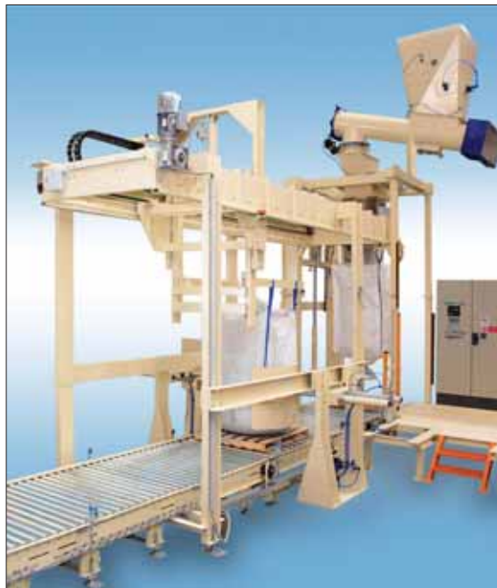
To overcome problems with fine powders like cement, CBC designed a system to provide continuous support for the loops at the filling point and during transfer to a second deaeration position
