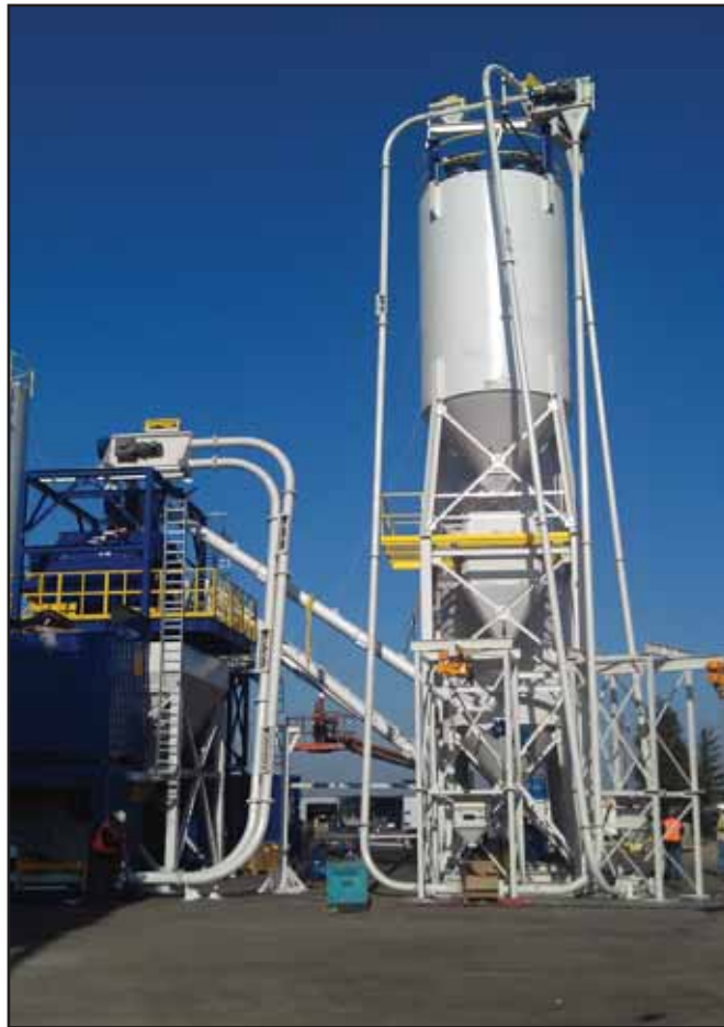
Spiroflow's ATEX compliant conveyors, bulk bag dischargers and fillers incorporate flow promotion devices to aid the movement of difficult materials with negligible degradation
