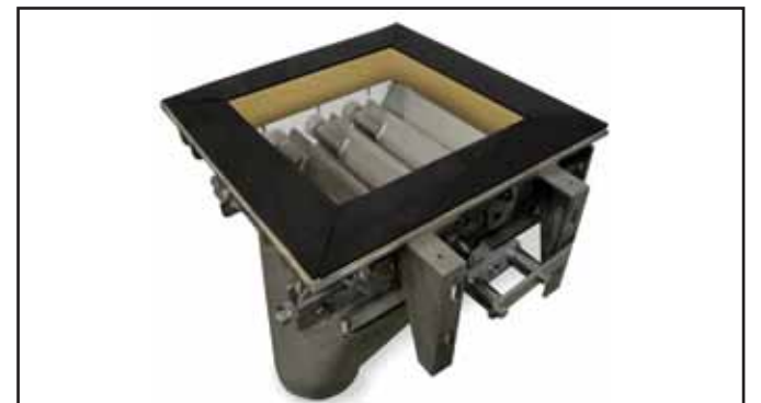
The bin activator has integral vibrating blades to maintain a steady momentum and minimise bridging
