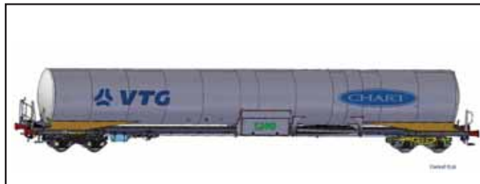
The prototype rail tanks will be capable of transporting double the payload of an LNG tank container or truck
