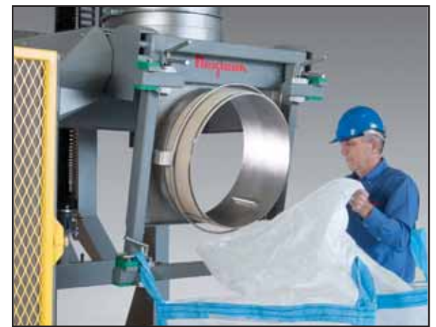
The Swing-Down fill head with wide-diameter spout seal allows safe, rapid connection of wide diameter bag spouts for passage of filter cake, aggregates, metal powders, abrasive minerals, dry chemical additives and irregular bulk materials
