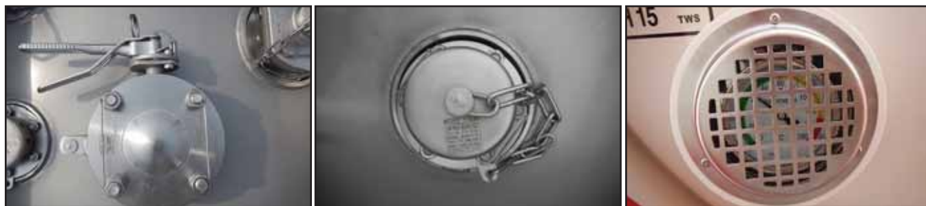
TWS H2O2 tank containers feature (from right to left) top discharge, a breather device and thermometer
