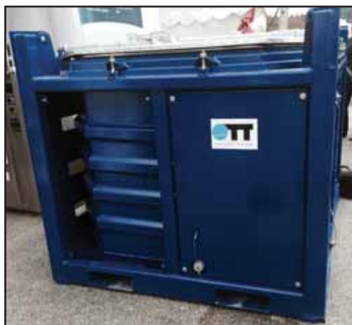
The heated mud container heats the contents sufficiently to allow emptying
