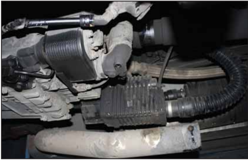
Mouvex B200 Series Flow Control Screw Compressor with special check and relief valve
