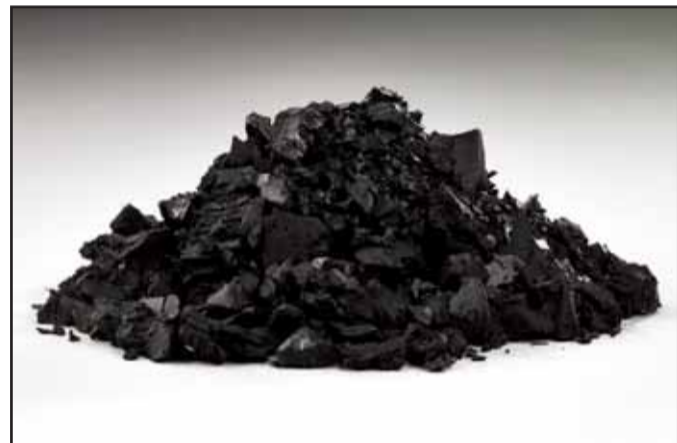
Rough ground particles from shredded scrap tyres comprise 80% of Edge Rubber's raw material
