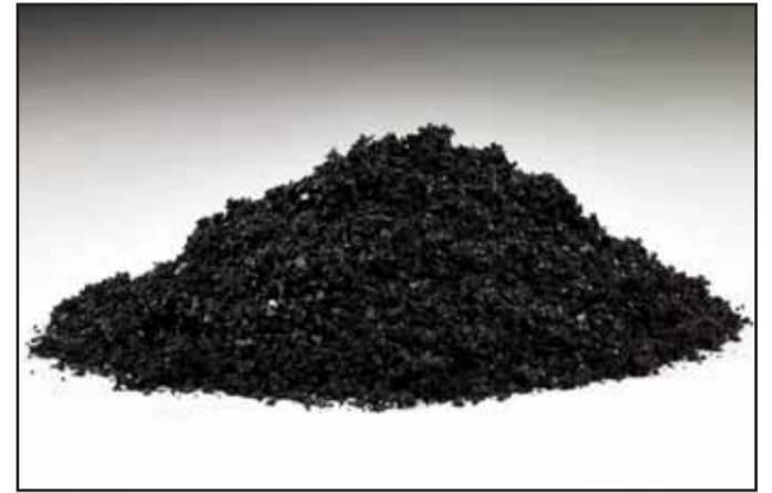
Crumb rubber particles that have been ground in the cracker mills are packaged for shipment to customers or conveyed to the micro milling process for reduction to the finest powders
