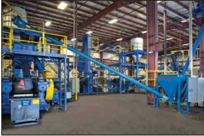
From the large hopper, two flexible screw conveyors transport ground rubber particles from the cracker mills to wet grind mills for the finest size reduction. Discharge chute (black) deposits the cracker mill grindings into the hopper
