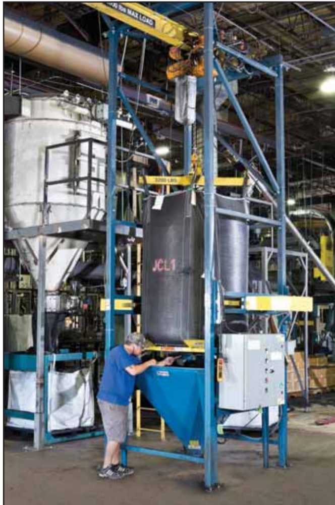
Bulk bag discharger and flexible screw conveyor feed rough ground particles and rubber buffings to cracker mill. The bulk bag is loaded into the discharger frame by electric hoist and trolley suspended from a cantilevered I-beam. The wide frame accommodates open-bottom design bags
