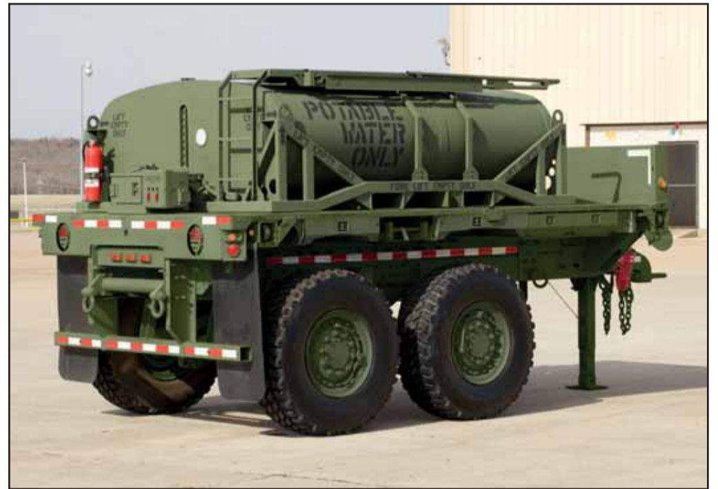
Camel tank – a 2000 litre LMV (light vehicle module) as supplied to the US army
