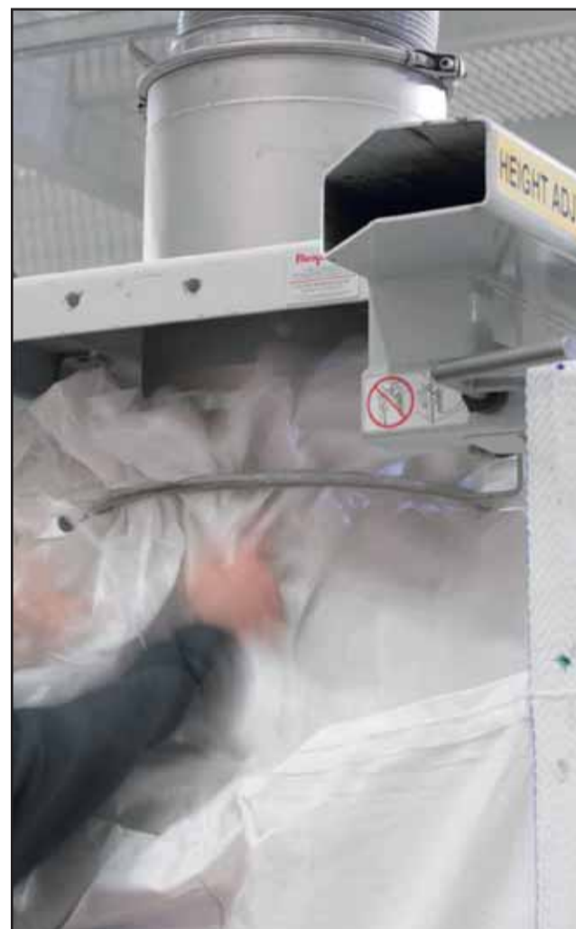
Bag spout is pulled over an inflatable collar which, together with a filtered air displacement vent, assure dust-free filling
