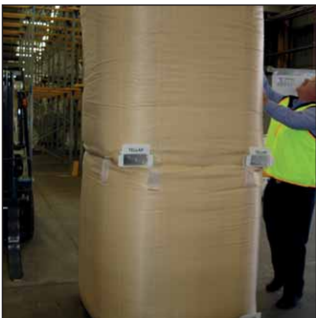
High strength sleeves are integrated into the base of the Tellap bag to replace the pallet, allowing a standard forklift truck to raise the bag from the base
