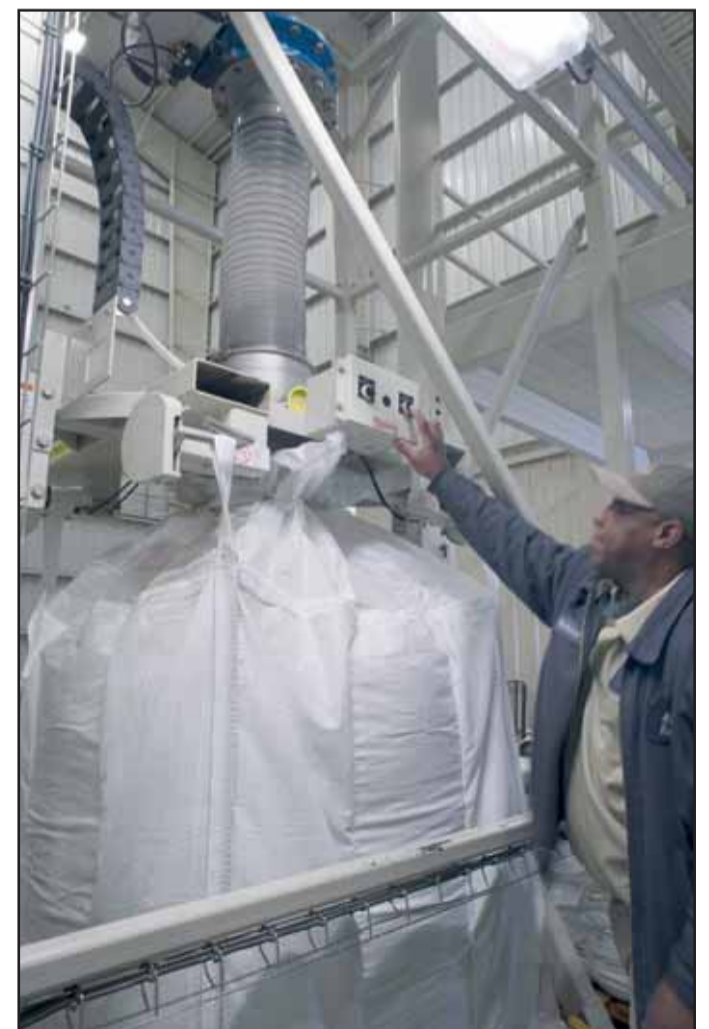
Operator inflates the bag, removing creases prior to filling
