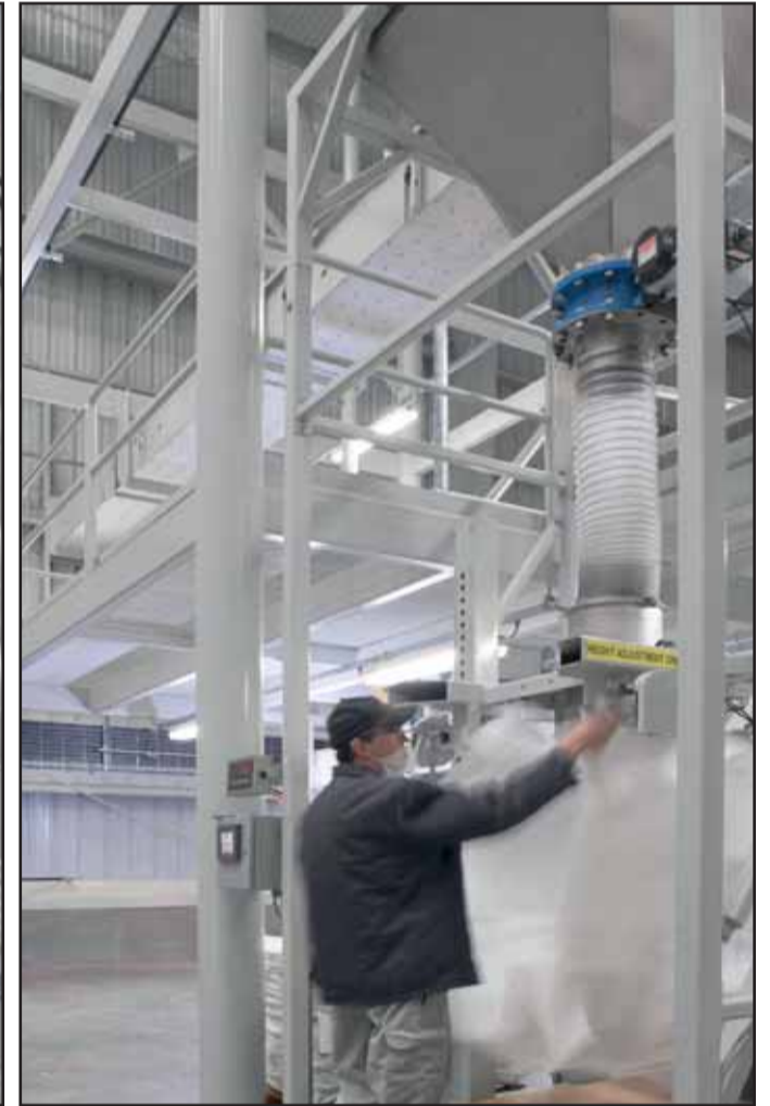
Operator attaches bag loops to retractable bag hooks that suspend the bag during filling
