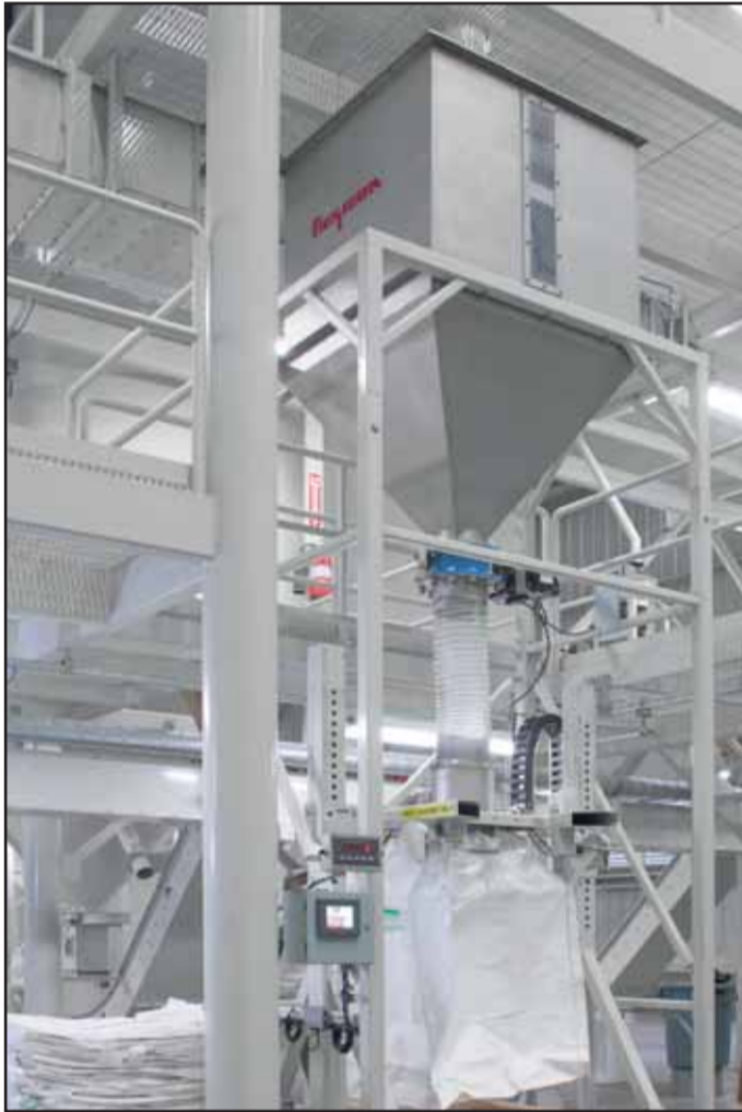
Rice descends from the hopper, through a dome valve and downspouting into the twin-centrepost bulk bag filler
