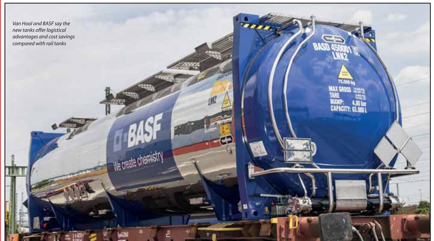
At 63 cbm and maximum allowable weight of 75 tons, Van Hool's 45ft container for BASF has a loading capacity double that of a conventional tank
