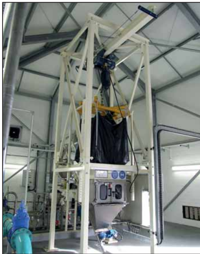
On assessing the customer's factory lay-out, Spiroflow designed an enclosed conveying system to maximise floor space at the plant using the T6 bulk bag discharger
