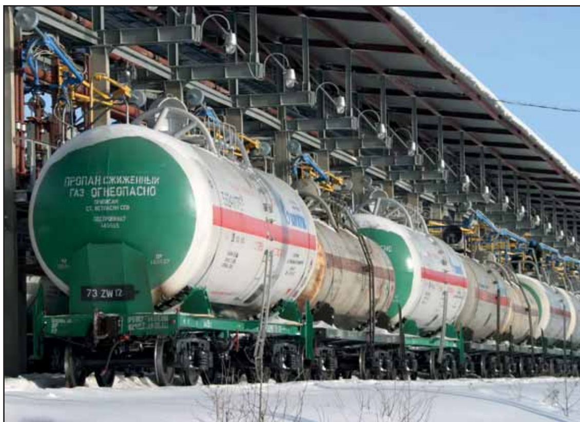
Loading facilities at many production plants were constructed for rail tanks, not containers, and require modification
