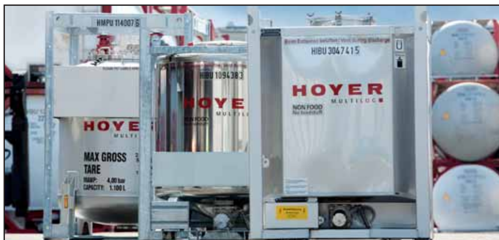
Adding type UN T 22 containers to its range means Hoyer is augmenting its own IBC fleet with a variant that makes high operating pressure levels possible
