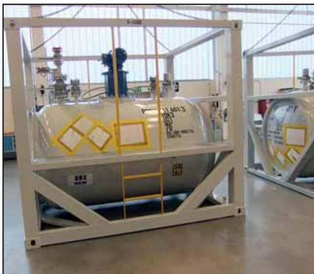
WEW's solution for Dow involved a 5,000 litre tank inside an ISO style frame fitted with a special agitator
