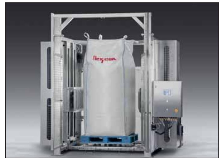
Flexicon's Block-Buster conditioner features hydraulically-actuated rams that automatically adjust in height for conditioning of short to extra-tall bulk bags, while reducing height of the loading deck by about 50 percent
