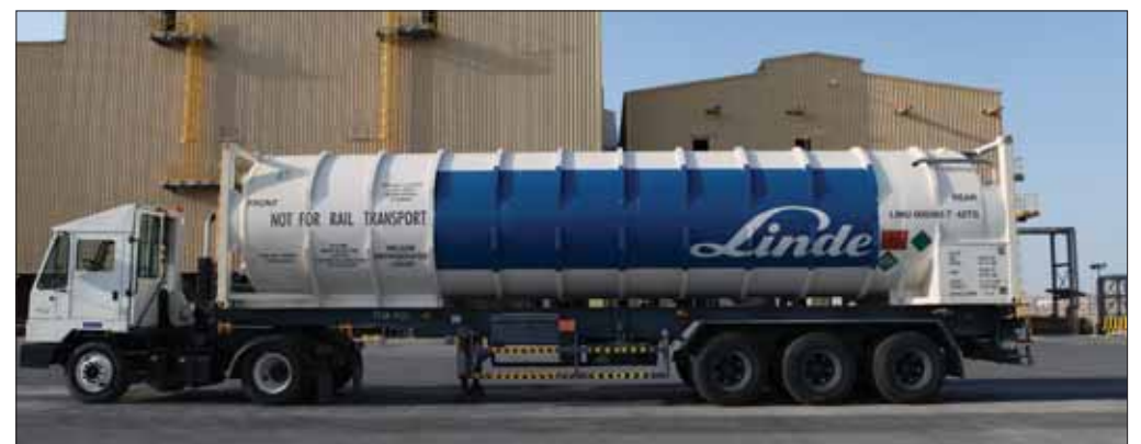
The helium containers can each hold some 41,000 litres
