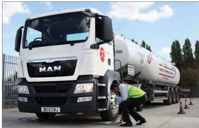
A Michelin Technical Manager performs a vehicle weighing exercise ahead of the trial to determine optimum inflation pressures.
