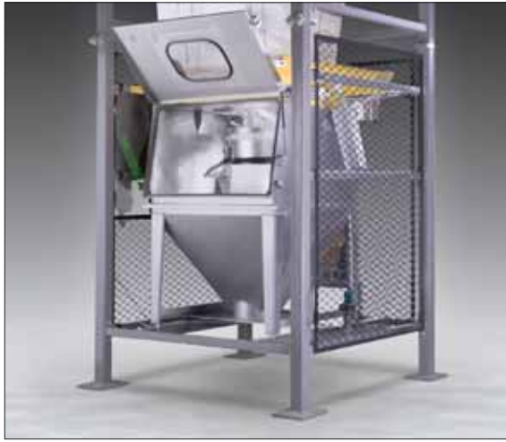
Flexicon's new Dust Hood contains material dislodged from folds in the bag spout during connection and disconnection, as well as incidental leakage of fine powders through seams in the bag, while associated dust is vented to an optional dust collector or plant bag house
