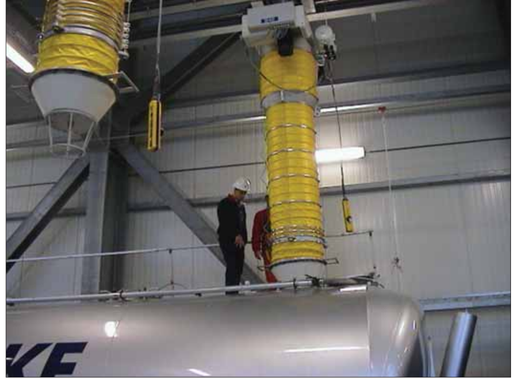
When loading into tanker trucks the chute outlet, the tight connection between chute outlet and hatch ensures a dust free loading process
