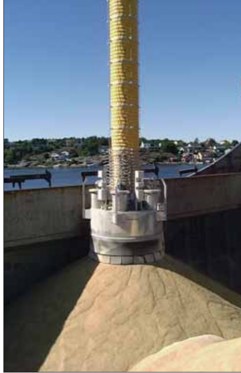
The chute outlet has integrated fully self-contained filter modules for minimising the dust emission from the product pile
