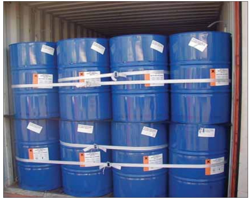
Cordstrap provides solutions for properly securing cargoes in containers
