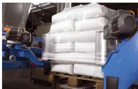
An RKW Group stretch hooding machine showing mechanical fingers applying a hood to palletised sacks
