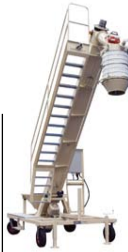
Van Beek Dino fitted with lump breaker and a sampler which can be manual or automatic
