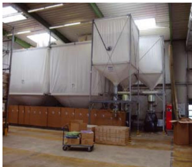
A key attraction of the A.B.S. flex-silo concept is that the storage facilities can be easily relocated; the silos pictured are storing EPS
