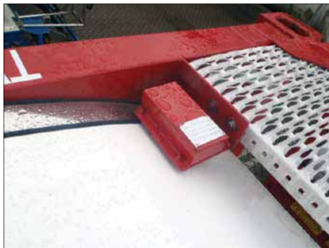
TWS came up with a GPS solution comprising a tamper-proof, battery-operated positioning system attached to the containers
