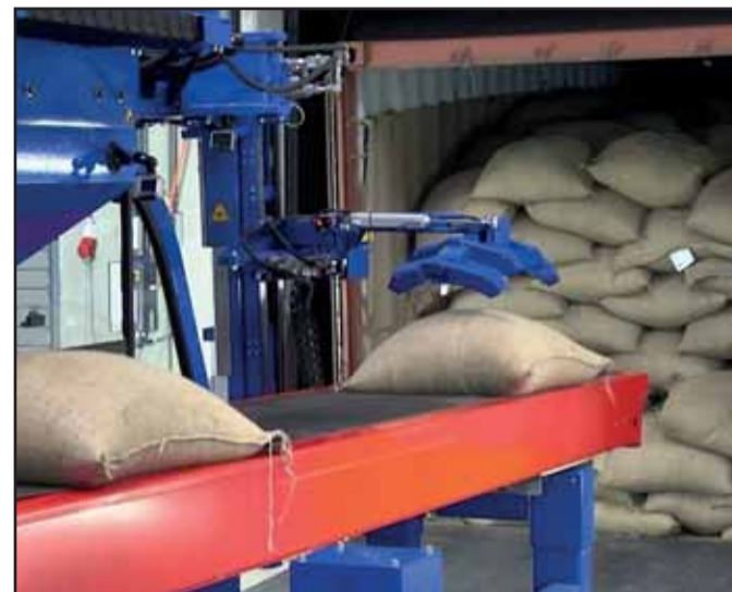
The bag line reduces heavy physical work when unloading and palletising bags out of containers
