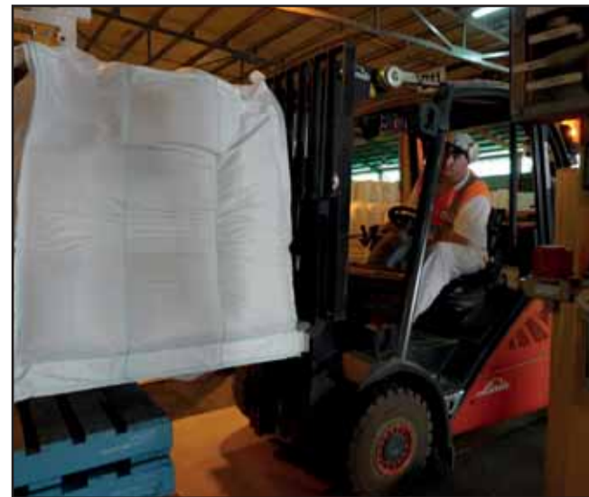
The Tellap bulk bag weighs only 5kg against up to 35kg for a conventional wooden pallet. High strength sleeves are integrated into the base of the bag to replace the pallet, allowing a standard forklift truck to raise the bag from the base
