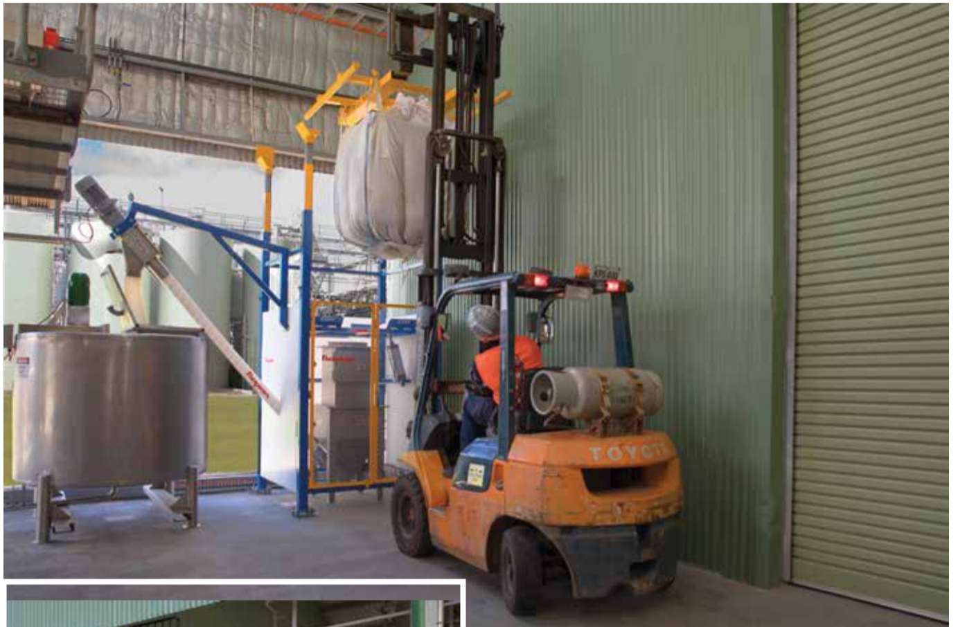
Above: Operator secures bag to the lifting frame with Z-Clip bag strap holders, and then loads the frame and bag onto the main discharger frame
