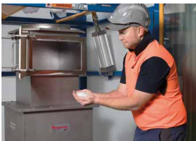
Operator pulls the bag spout into the bulk bag interface chute and unties the drawstring. A sealing ring, dust-tight door and filter sock contain dust
