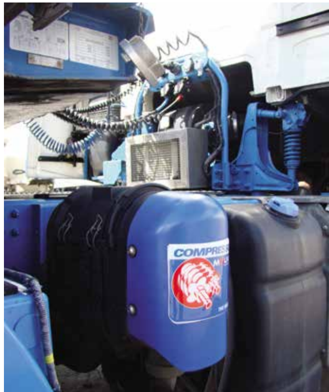
The compact size and light weight (110kg) of the MX12 allows it to fit easily within the truck frame
