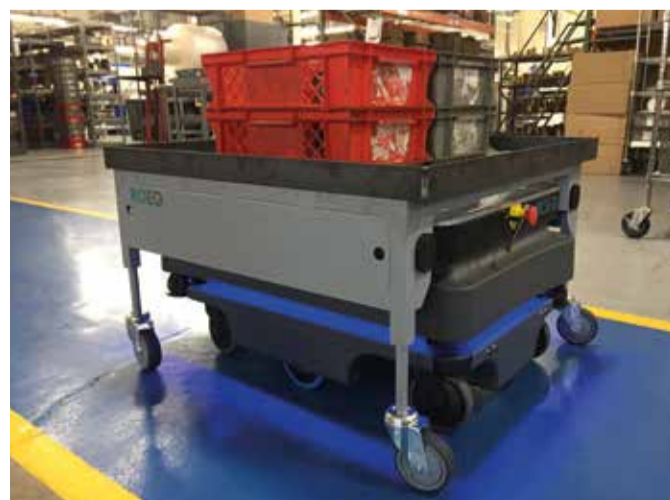
Inpro/Seal will use robotic tuggers to move raw materials around the facility
