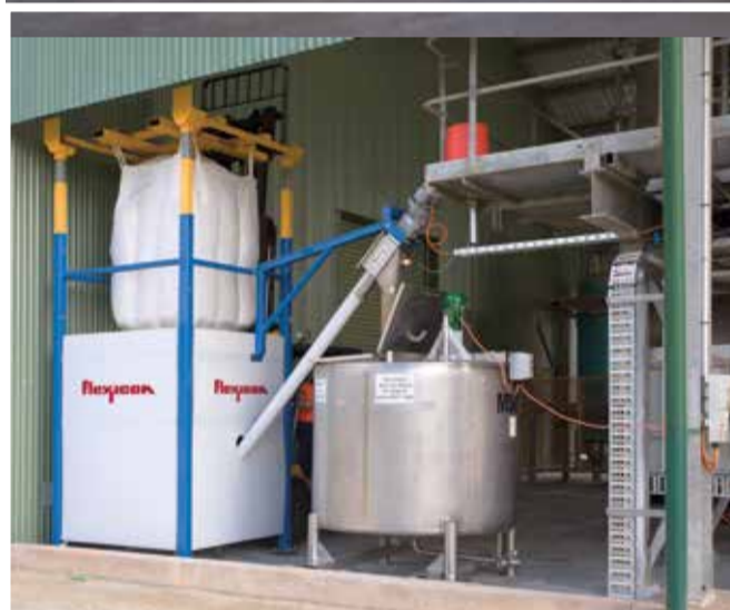
Above: Operator secures bag to the lifting frame with Z-Clip bag strap holders, and then loads the frame and bag onto the main discharger frame
