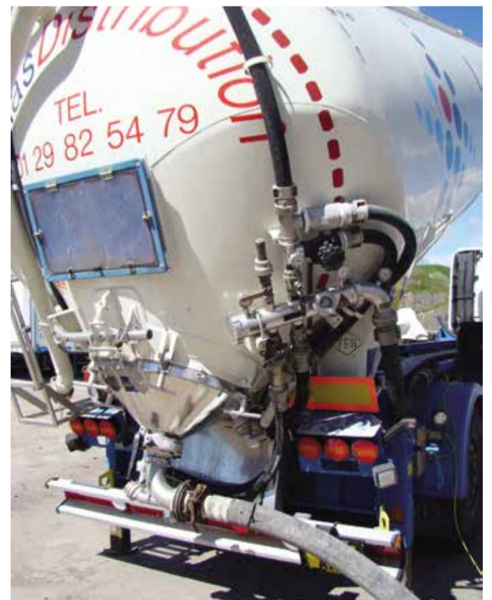
The ability of the MX12 to create two bars (29 psi) of air pressure is critical when unloading dry-bulk products
