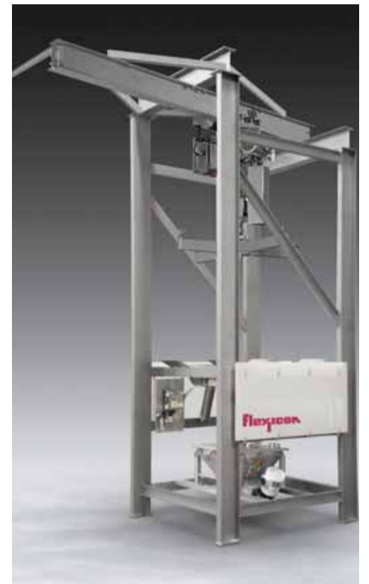
The open-channel stainless steel construction of the Flexicon bulk bag discharger eliminates internal voids where contamination can breed, and allows rapid sanitising and inspection.
