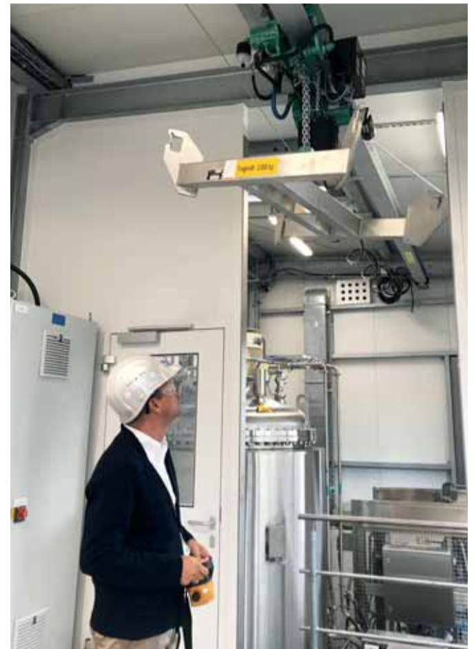
The JD Neuhaus Profi 2 T1 hoist in low headroom trolley, ideal for use where headroom is restricted
