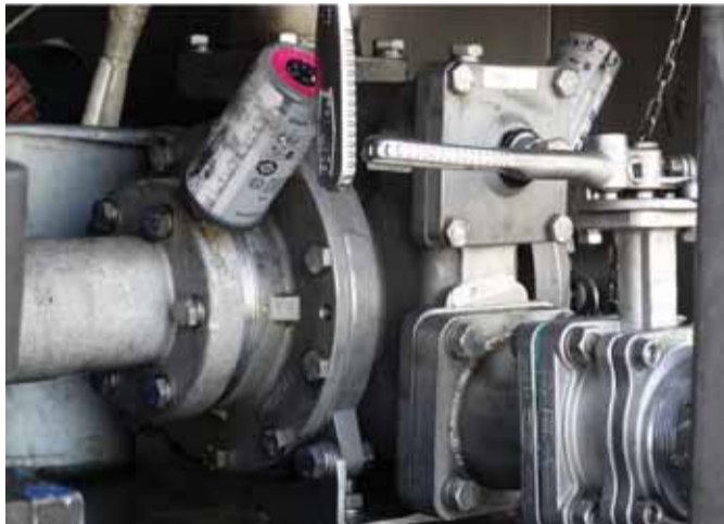
Blackmer STX Series Sliding Vane Pumps feature a 316 stainless-steel body and internals with chemical-resistant seals, bearings and O-rings, all of which make it an ideal solution when transferring corrosive liquids like hydrogen peroxide
