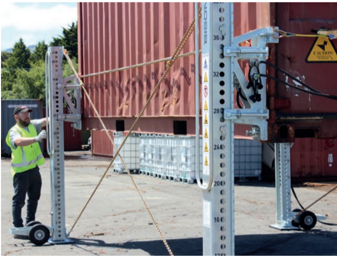
The P Series handles containers weighing up to 32 tonnes
