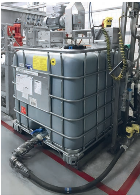
The Schütz IBC with the Impeller and agitator drive is directly connected to the production line with a 2ins camlock
