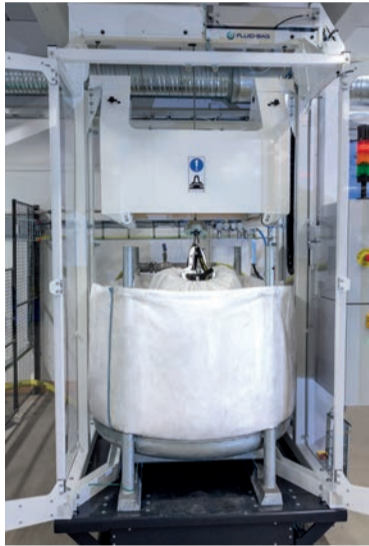
A Fluid-Bag in the automatic discharge roller
