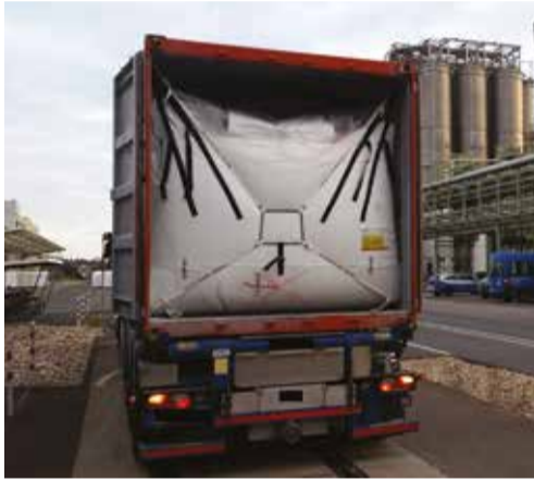
The Barless Safety System was developed to address the lack of standardisation about steel bars used to secure the bulkhead area
