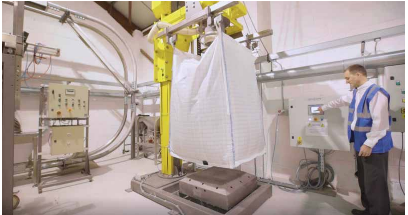
Spiroflow's CTE bulk bag filler features the cone table densification system which densifies material in the bag, increases bag stability and bulk bag filling throughput
