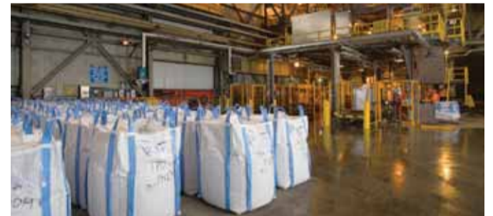
The automated bulk bag filling system includes two bulk bag fillers, a central pallet dispenser, and two 25ft long roller conveyors from which a fork truck offloads filled bags for shipment
