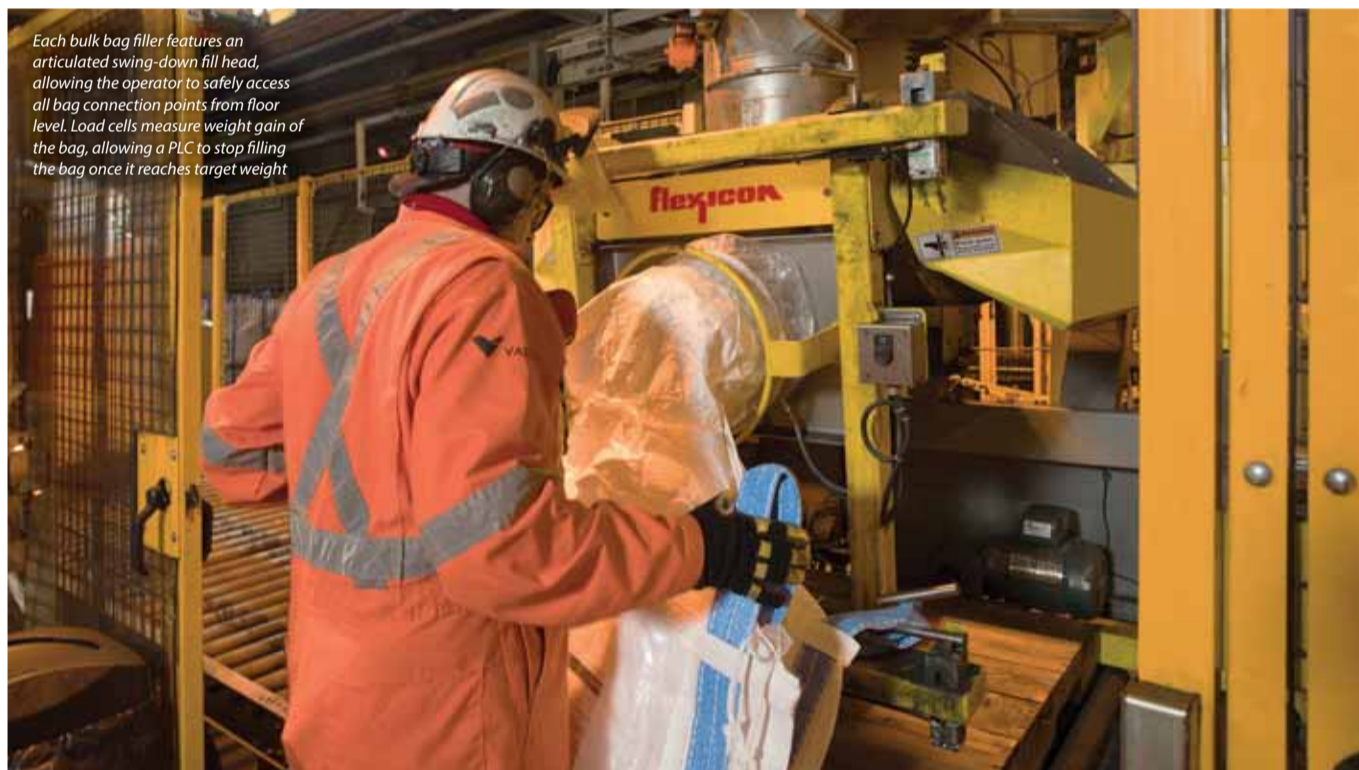
The automated bulk bag filling system includes two bulk bag fillers, a central pallet dispenser, and two 25ft long roller conveyors from which a fork truck offloads filled bags for shipment
