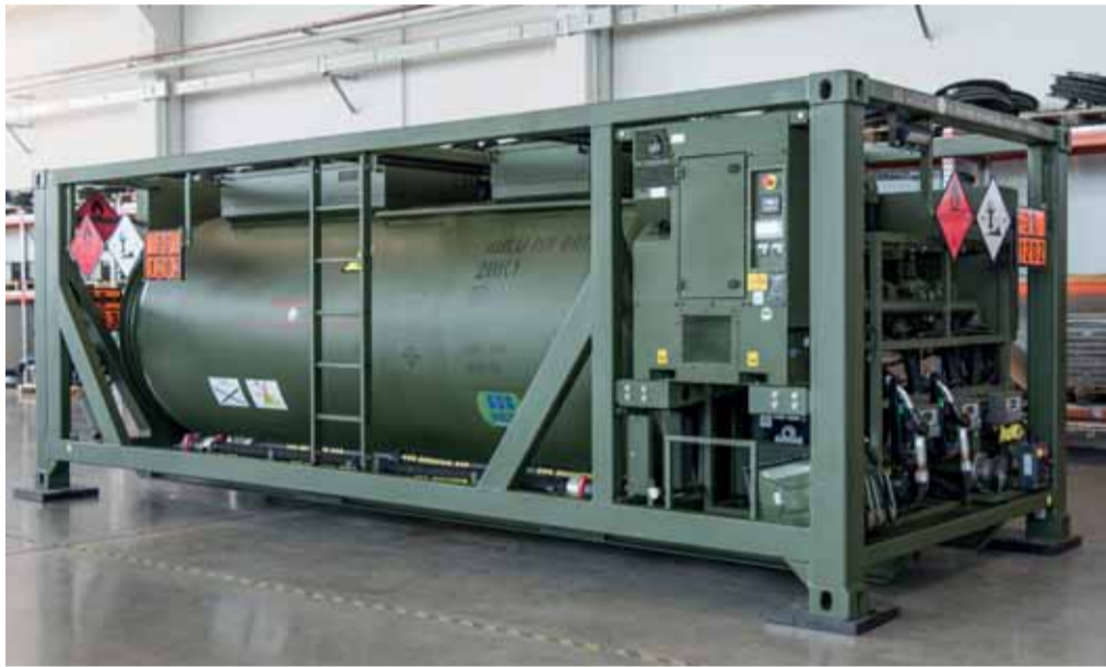
WEW developed an 8,000 litre fuel container to meet the Belgian Army's requirements
