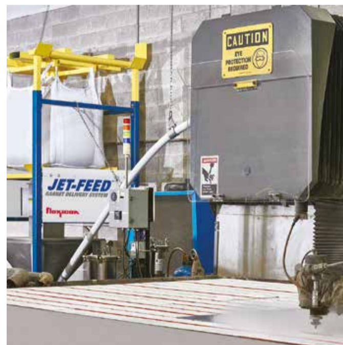
The system eliminates worker fatigue, potential injury, labour, spillage, dust, downtime and higher material cost associated with manual bag dumping
