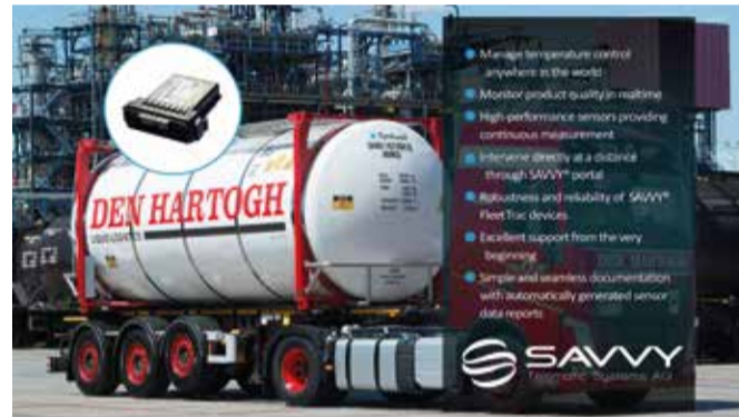
Data is sent by the telematic units to the Savvy Synergy software portal where Den Hartogh dispatchers can access them
