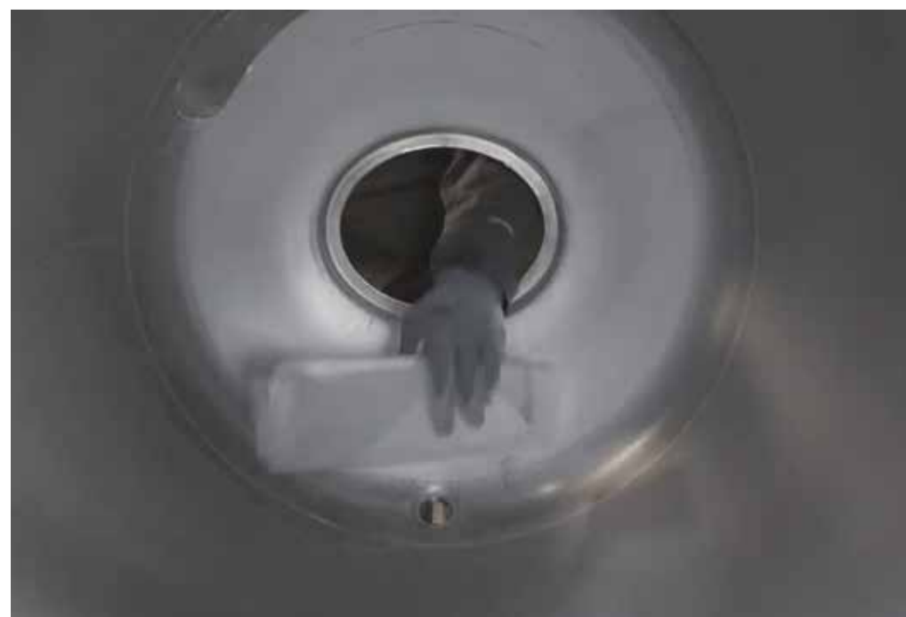
With the 'Bag-In-Tank' liner, draft beer is kept under pressure in the tank with compressed air instead of CO 2
