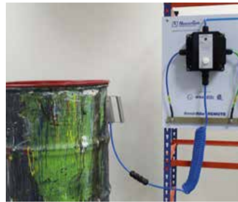
The VESX50-IP is fully compatible with Newson Gale's Bond-Rite and Earth-Rite monitoring systems
