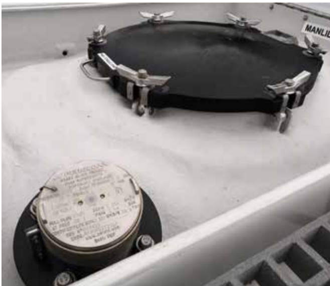
Composite tanks need specialised valves and fittings that can withstand the highly corrosive cargo
