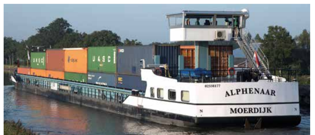
The Alphenaar is the first Dutch inland vessel to use interchangeable energy containers for propulsion
