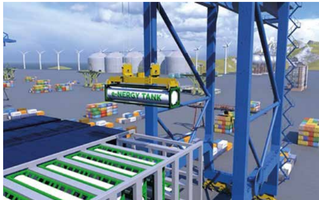
The capacity of each tank is 31 gross tonnes and about 33 cbm of LNG
