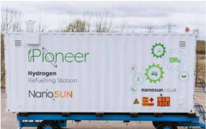
NanoSUN's Pioneer HRS combines volume gas storage, transport and end use vehicle dispensing in a single ISO container
