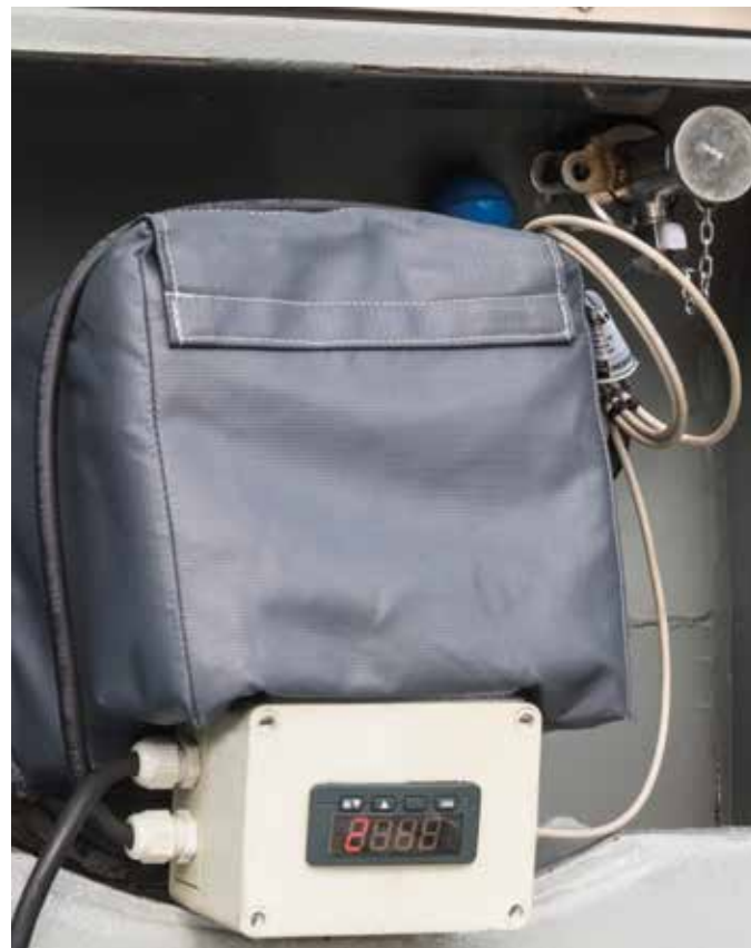
The heating sock's temperature can be set manually between 0 and 80 degrees, preventing product solidification around the product valve
