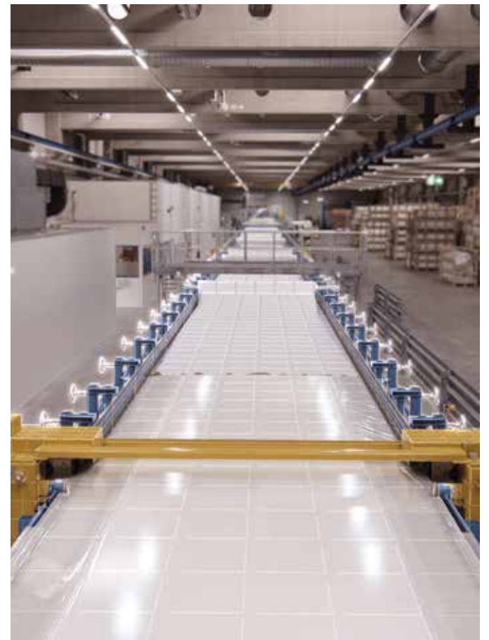
The fibre-reinforced composites are produced in a continuous, automated production process
