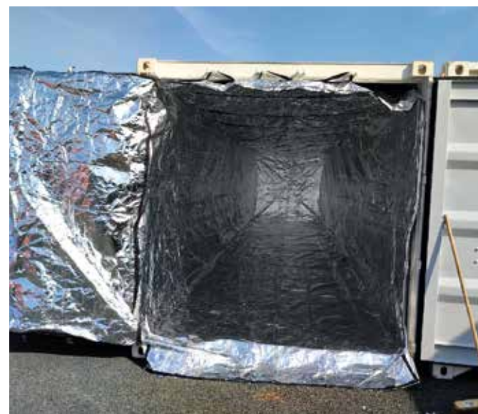
Using a thermal liner entails a fraction of the cost of using a reefer container, says BT Pack
