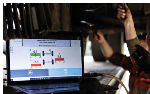
Readings are automatically measured by the Cam-aligner
